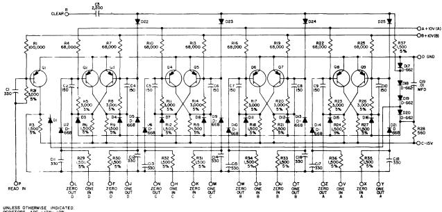
UNLESS OTHERWISE INDICATED: RESISTORS ARE 1/2W; 10% CAPACITORS ARE MMED TRANSISTORS ARE DEC 2094-4 DIODES ARE 0-664
