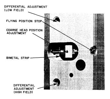
Figure 6-4 Read/Write Head Components
