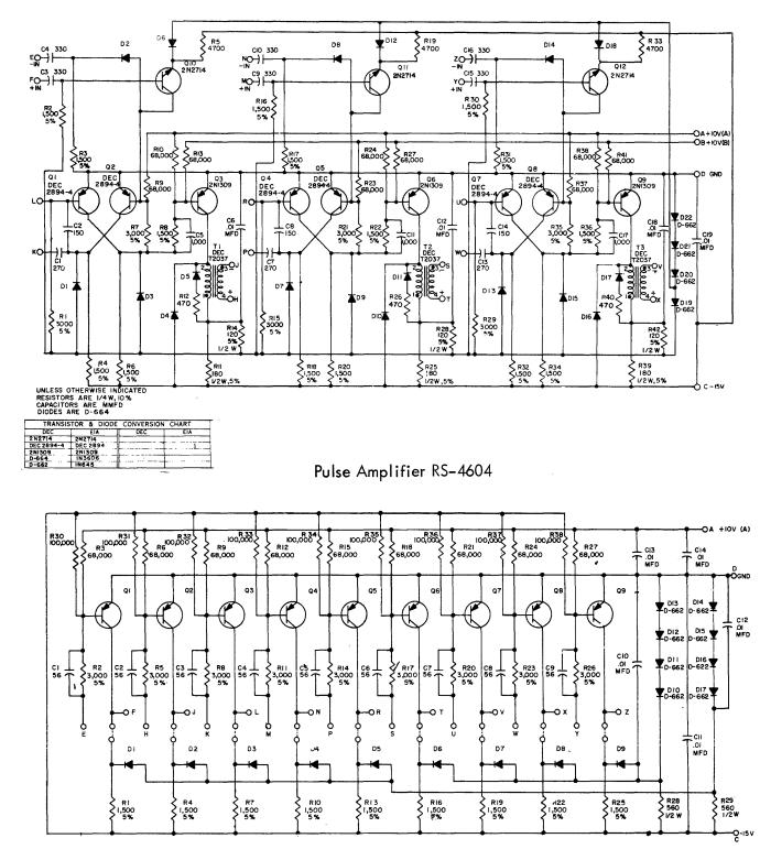
UNLESS OTHERWISE INDICATED RESISTORS ARE 1/4 W, 10 % CAPACITORS ARE MMFD TRANSISTORS ARE DEC 2894-1 DIODES ARE D-664
