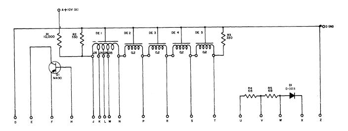
UNIESS OTHERWISE INDICATED: RESISTORS ARE 1/2W; 10% DEI= TECHNITROL 0.2µ90C DELAY LINE 330 OHMS TAPPED AT 0.05µ90C. INTERVAL DE2= DE5 TECHNTROL 0.2µ90C. DELAY LINE
