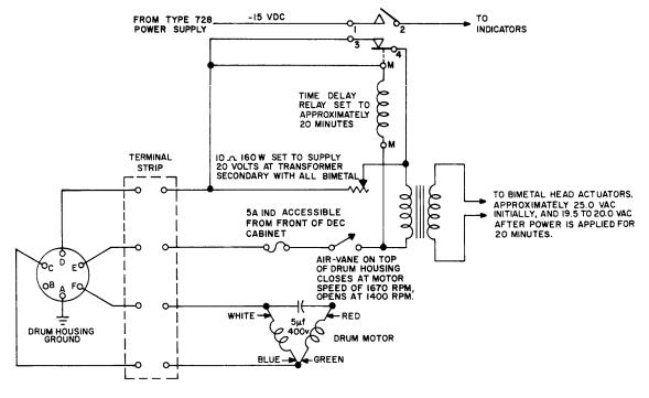
Figure 2-3 Drum Power Circuit
