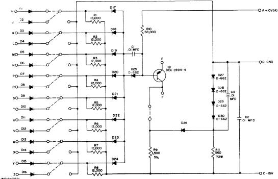
UNLESS OTHERWISE INDICATED: RESISTORS ARE 1/4W; 10% DIODES ARE D-664
