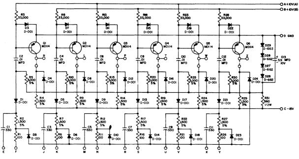
UNLESS OTHERWISE INDICATED: RESISTORS ARE 1/4W, 10% CAPACITORS ARE MMFD
