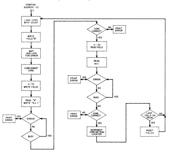
Figure A1-3 4096 Word Transfer Starting with Field Zero
