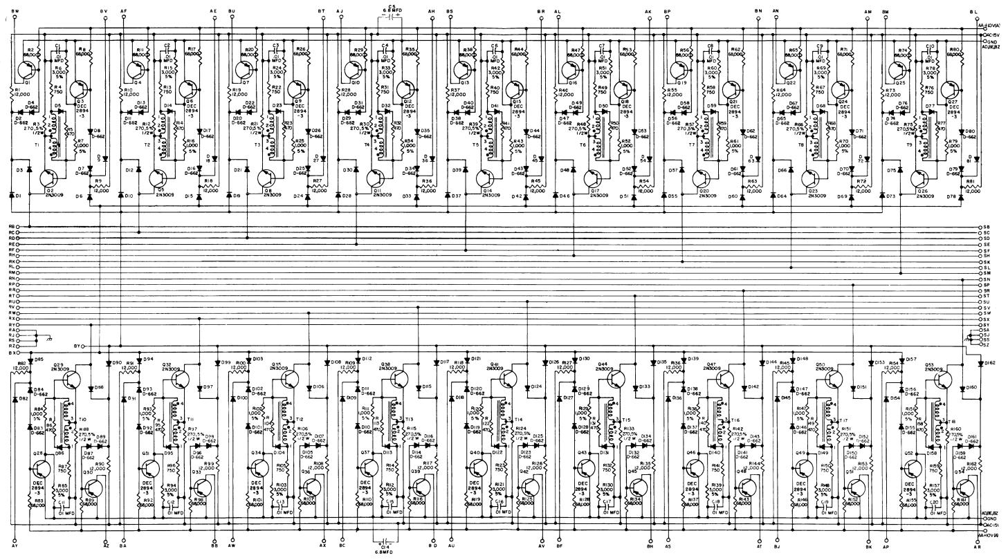
UNLESS OTHERWISE INDICATED: TRANSFORMERS ARE T-2044 DIODES ARE D-664 RESISTORS ARE I/4W, 10% TRANSISTORS ARE DEC 2894-1
