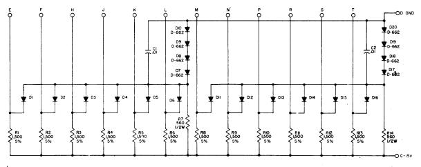
UNLESS OTHEWISE INDICATED: RESISTORS ARE 1/4W; 10% CAPACITORS ARE MFP DIODES ARE D-664
