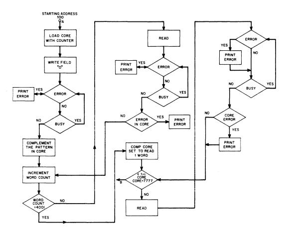
Figure A1-1 Parallel Drum Type 23 Test
