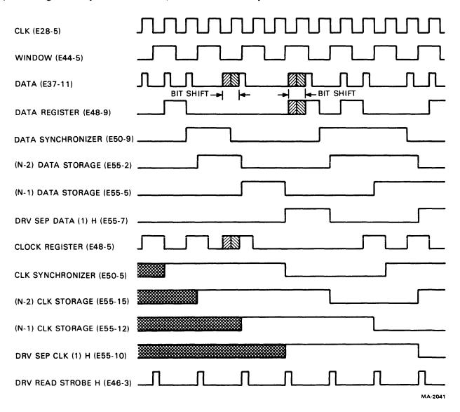
Figure 5-32 Data SYNC Timing Diagram
