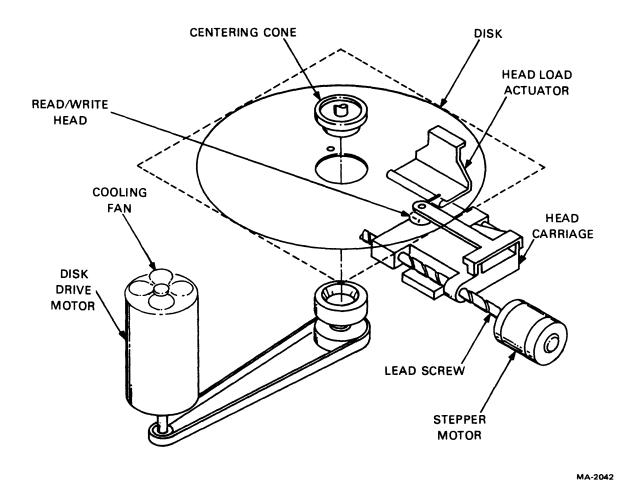
Figure 5-33 Disk Drive Mechanical System
