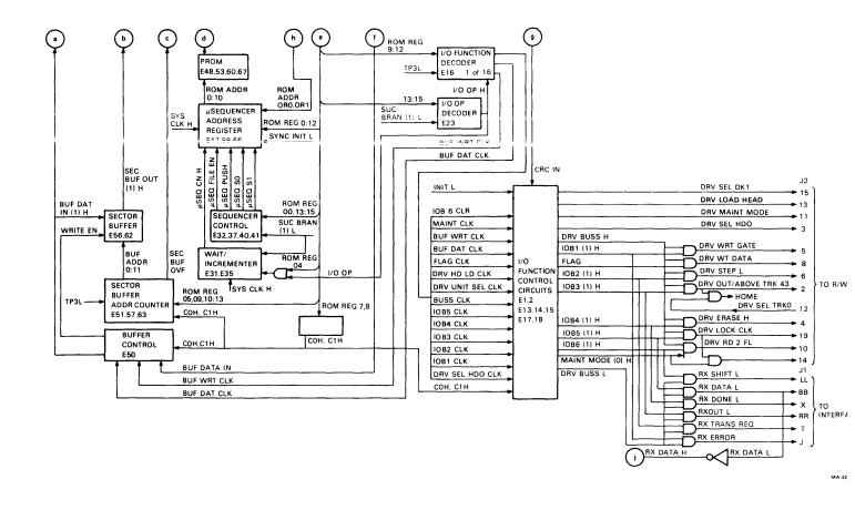
Figure 5-13 μCPU Controller Block Diagram (Sheet 2 of 2)
