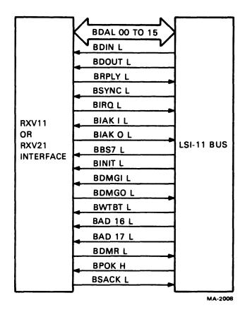
Figure 5-4 LSI-11 Bus to RXV11/RXV21 Interface Signals
