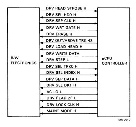
Figure 5-6 µCPU Controller to Read/Write Electronics Signals
