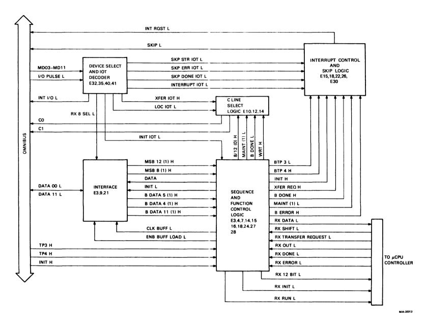
Figure 5-8 RX8E/RX28 Interface Block Diagram
