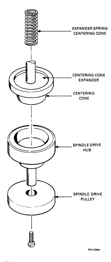
Figure 5-35 Centering Cone and Drive Hub
