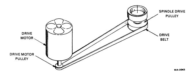
Figure 5-34 Drive Mechanism
