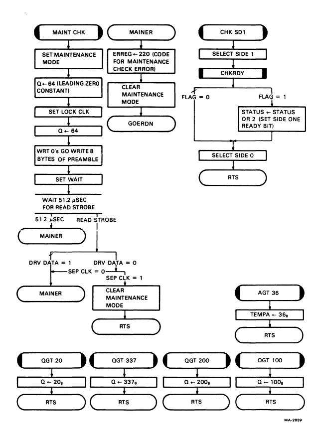
Figure 5-30 Maintenance Check Ready Subroutine Flowchart
