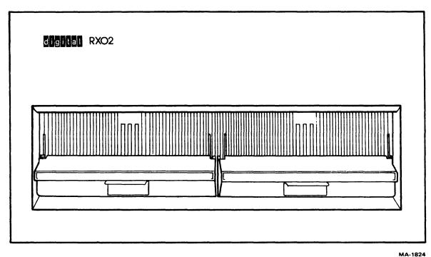
Figure 1-2 Front View of the Floppy Disk System
