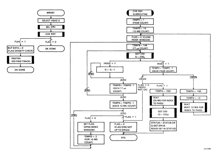
Figure 5-27 Maintenance Read Status and Check Ready Subroutines Flowchart
