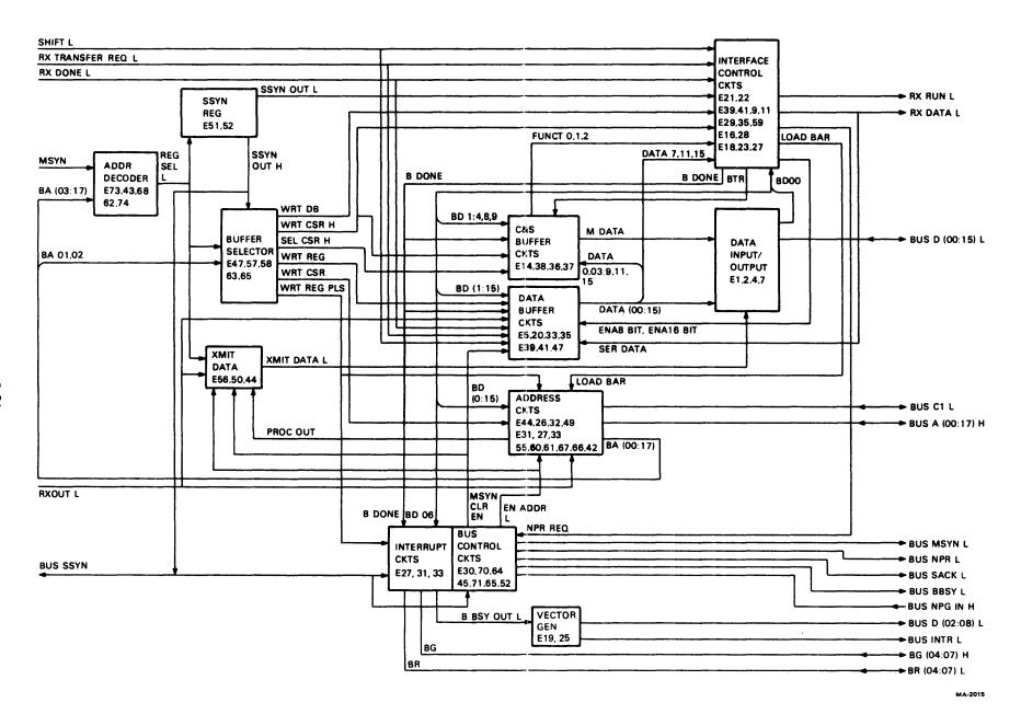
Figure 5-11 RX211 Interface Module Block Diagram
