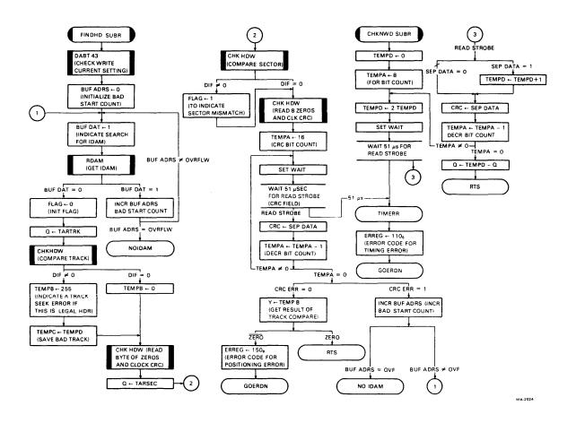
Figure 5-19 Find Header Subroutine Flowchart
