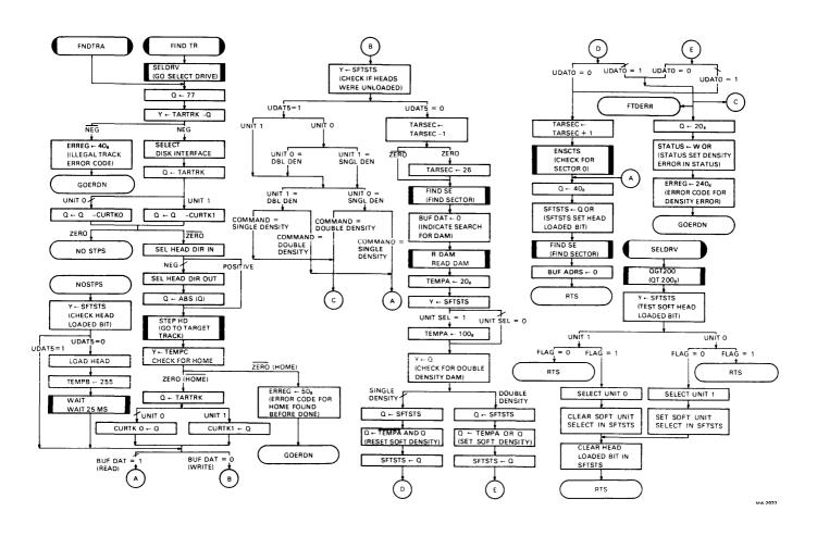
Figure 5-25 Select Drive and Find Track Subroutines Flowchart
