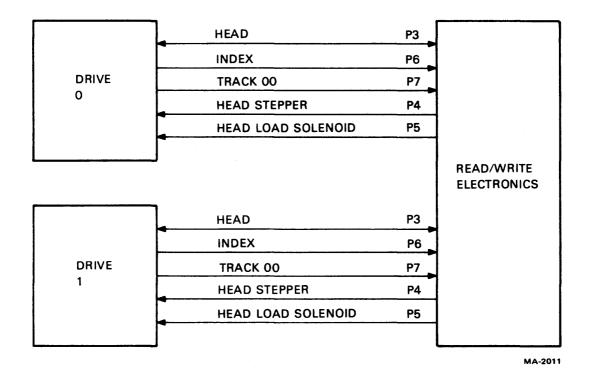
Figure 5-7 Read/Write Electronics to Drive Signals
