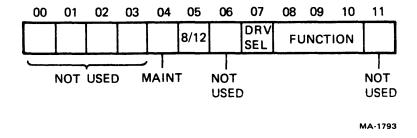
Figure 4-3 Command Register Format (RX8E)
