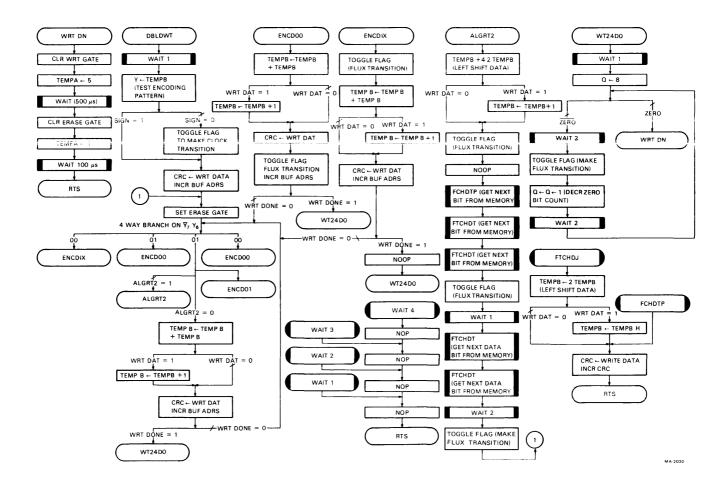
Figure 5-22 Write/Write Sector Subroutine Flowchart (Sheet 2 of 2)
