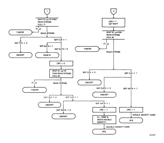
Figure 5-20 Read Address Mask Subroutine Flowchart (Sheet 3 of 3)
