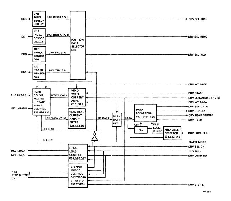
Figure 5-31 Read/Write Electronics Block Diagram
