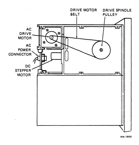
Figure 1-5 Underside View of Drive
