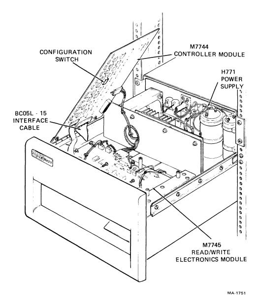
Figure 1-4 Top View of RX02
