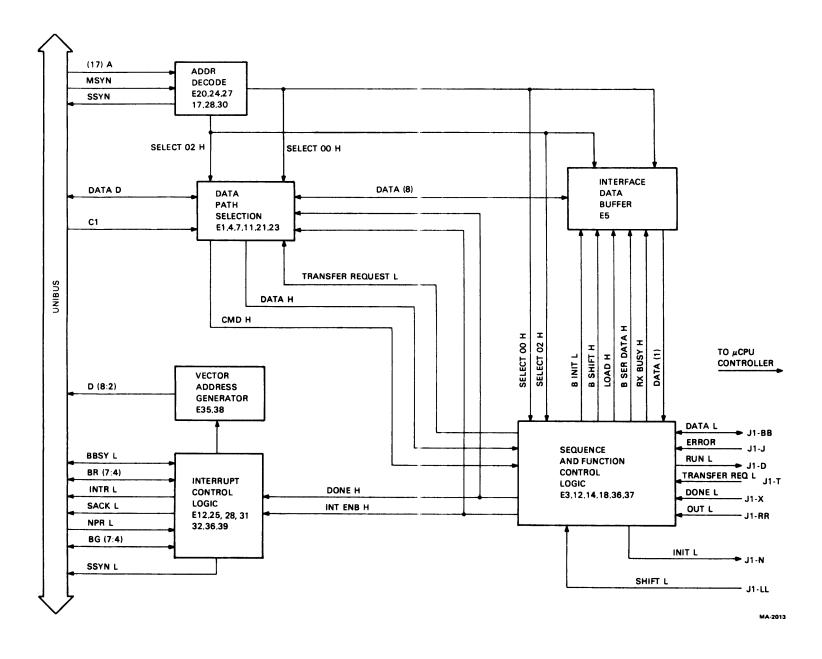
Figure 5-9 RX11 Interface Block Diagram
