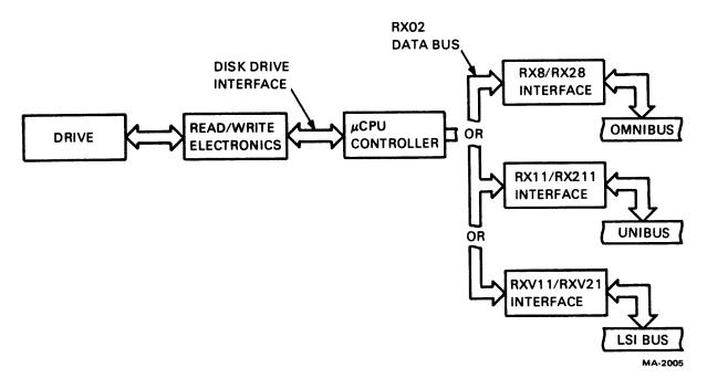
Figure 5-1 RX02 System Block Diagram
