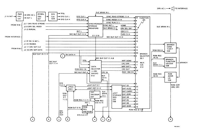
Figure 5-13 μCPU Controller Block Diagram (Sheet 1 of 2)
