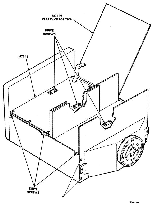
Figure 6-1 RX02 Component Location Diagram
