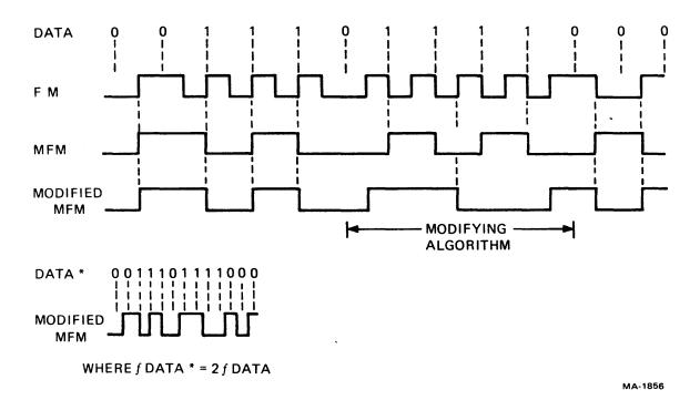
Figure 1-8 FM Versus MFM Encoding
