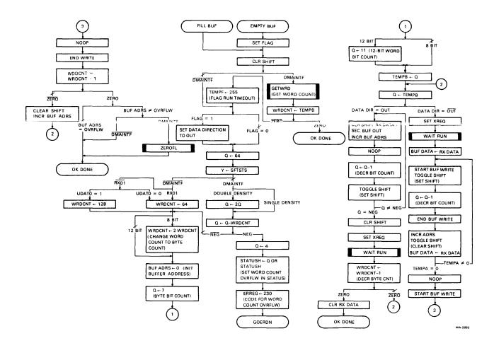
Figure 5-24 Fill/Empty Buffer Routine Flowchart
