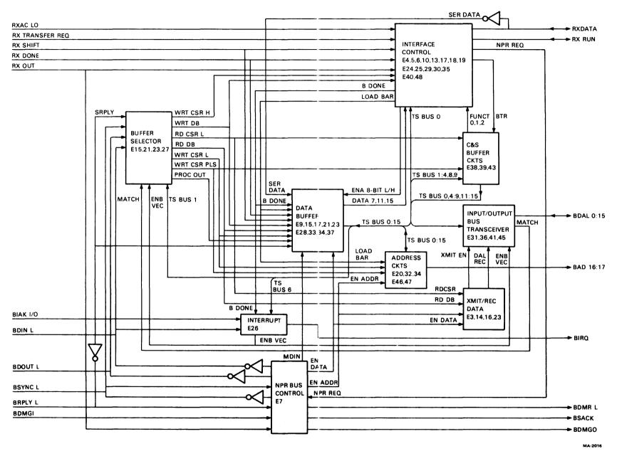
Figure 5-12 RXV21 Interface Module Block Diagram
