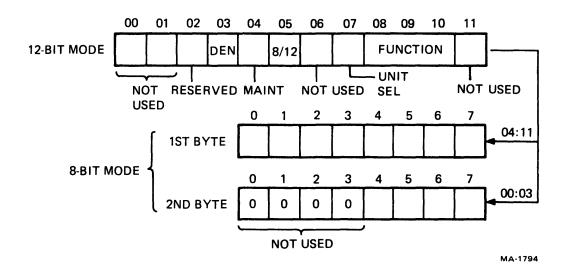
Figure 4-4 Command Register Format (RX28F)
