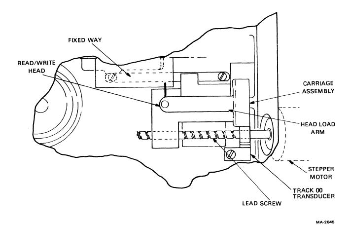
Figure 5-36 Positioning Mechanism
