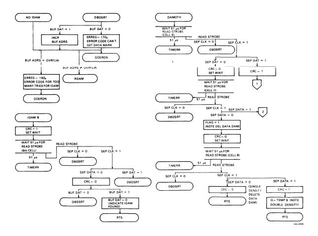
Figure 5-20 Read Address Mask Subroutine Flowchart (Sheet 2 of 3)
