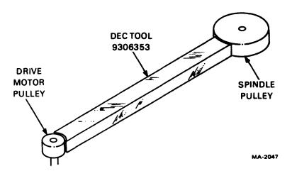
Figure 6-2 Drive Motor Positioning Diagram
