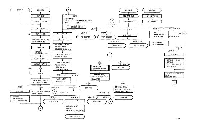
Figure 5-26 Decode Command Routine Flowchart (Sheet 1 of 2)
