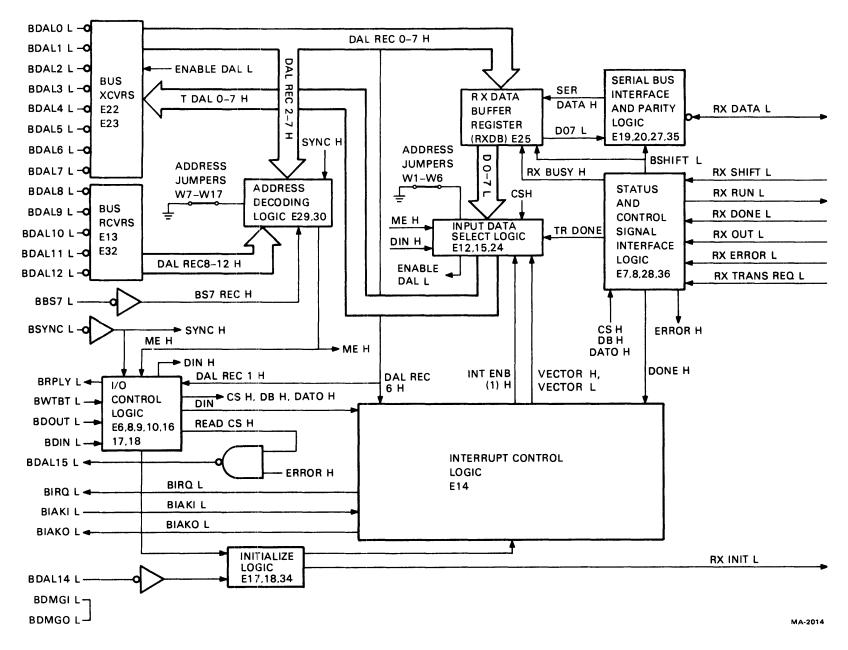
Figure 5-10 RXV11 Interface Block Diagram
