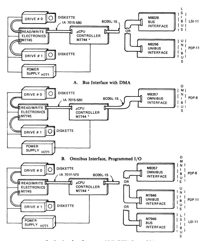
C. Bus Interface, Programmed I/O (RX01 Compatible)
