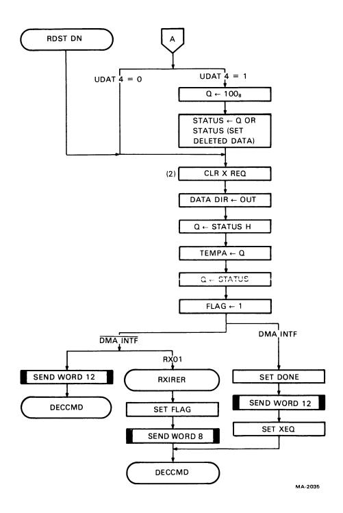
Figure 5-26 Decode Command Routine Flowchart (Sheet 2 of 2)
