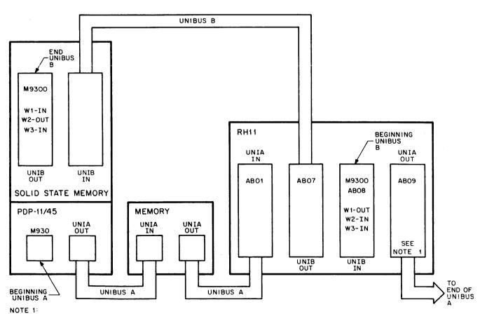
Install M930 terminator if last device on UNIBUS A.
