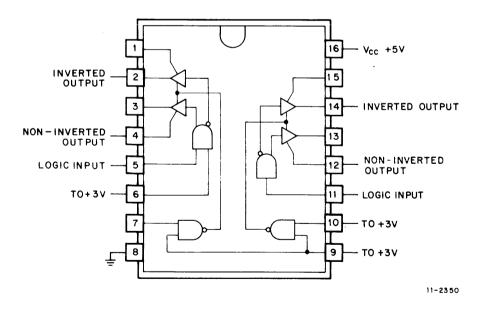
Figure 6-9 Dual Differential Driver Pin Connection Diagram
