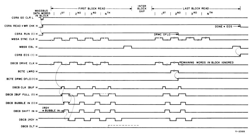
Figure 6-4 Read & Write Check MASSBUS Timing Diagram
