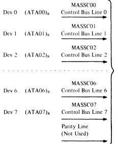
Asynchronous Control Bus (Total of 17 lines) The controller strobes the eight Attention Active (ATA) bits from the asynchronous control bus 1  $\mu$ s after placing the RPAS address on the Register Select lines to see the results of the Attention Summary request.
