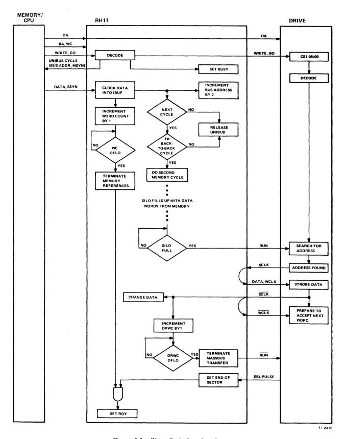
Figure 5-5 Write Cycle Interface Diagram
