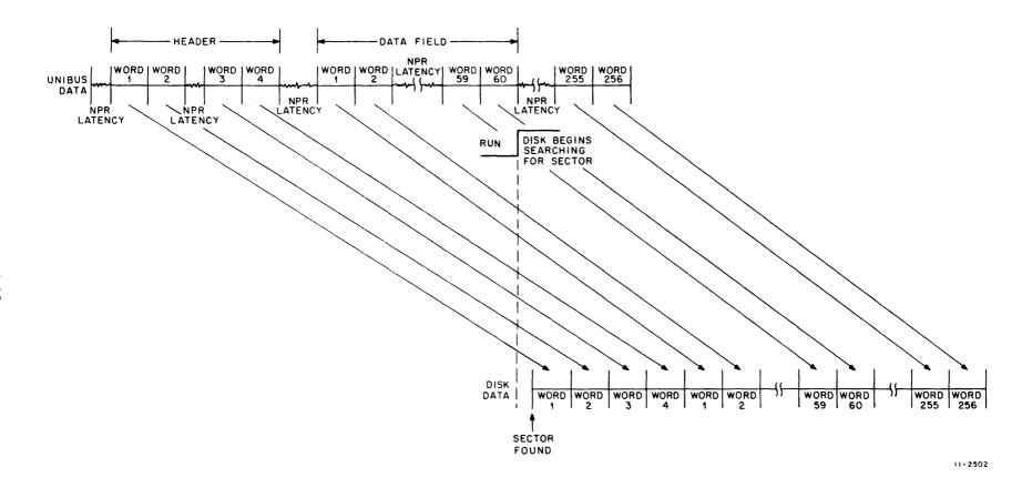
Figure 1-10 Write Header and Data Command Transfer (Pack Format Command)
