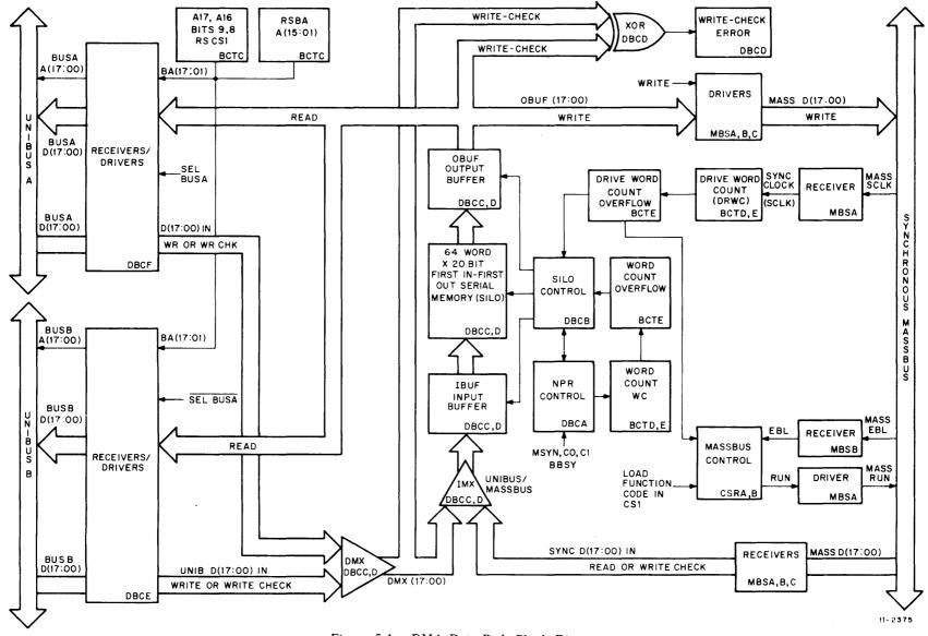
Figure 5-4 DMA Data Path Block Diagram
