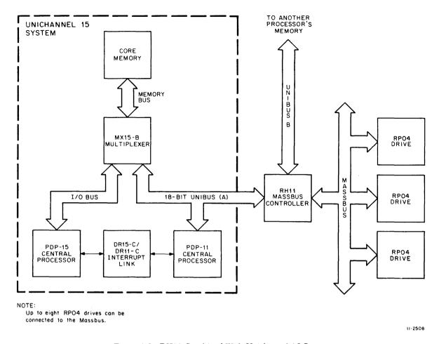
Figure 1-3 RH11 Combined With Unichannel 15 System
