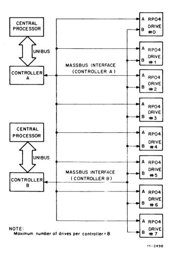
Figure 3-6 Dual-Controller Configuration
