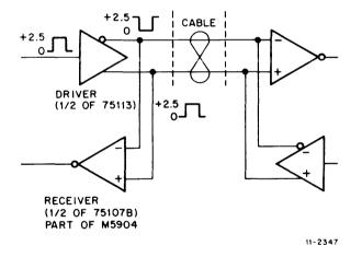
Figure 6-6 Typical Differential Driver/Receiver Connection
