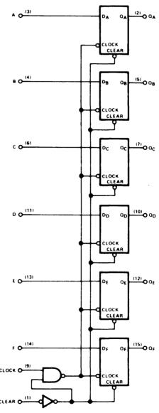
$Pin (16) = V_{CC}, Pin (8) = GND$
