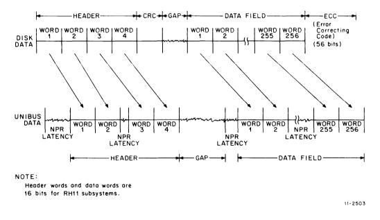
Figure 1-9 Read Header and Data Command Transfer
