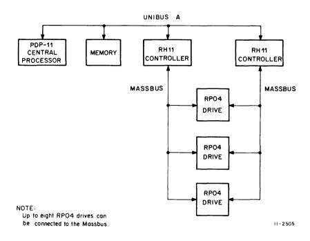
Figure 1-4 Dual Controller Option (With One Processor)
