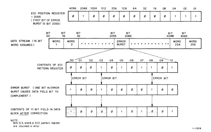
Figure 3-7 Example of Error Correction Process
