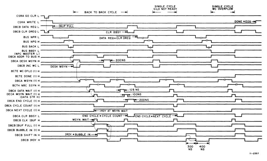
Figure 6-1 Write UNIBUS Timing Diagram
