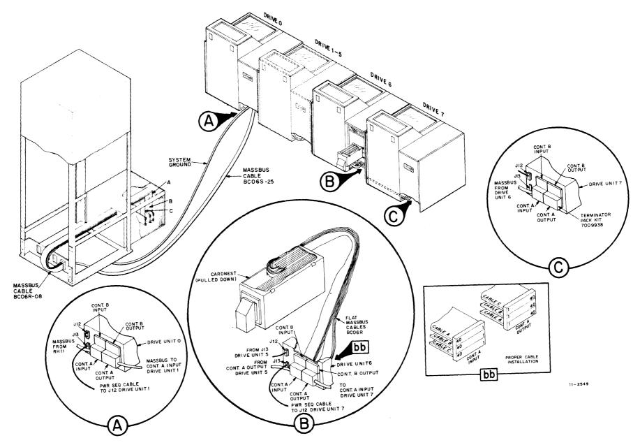
Figure 2-2 Single-Port Subsystem Cable Routing
