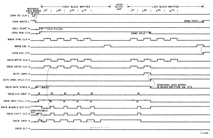
Figure 6-3 Write MASSBUS Timing Diagram
