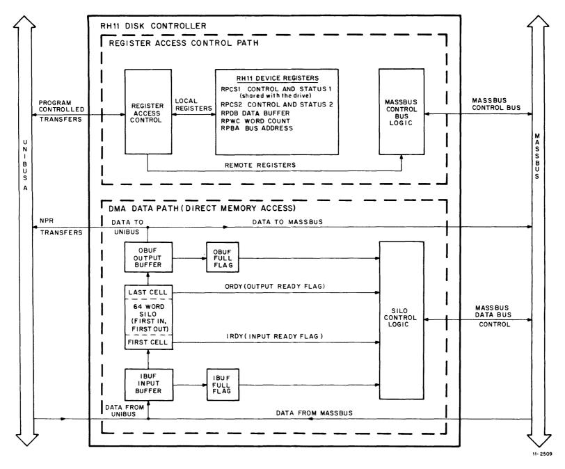
Figure 1-6 RH11 Simplified Data Path Diagram
