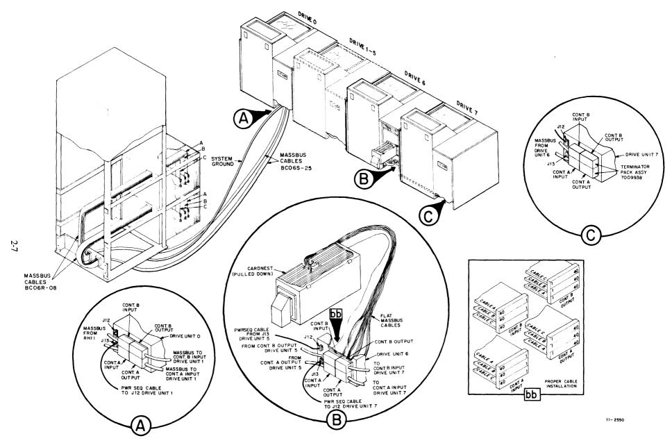
Figure 2-3 Dual-Port Subsystem Cable Routing
