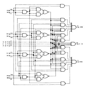
Pin (16) =  $V_{CC}$ , Pin (8) = GND
