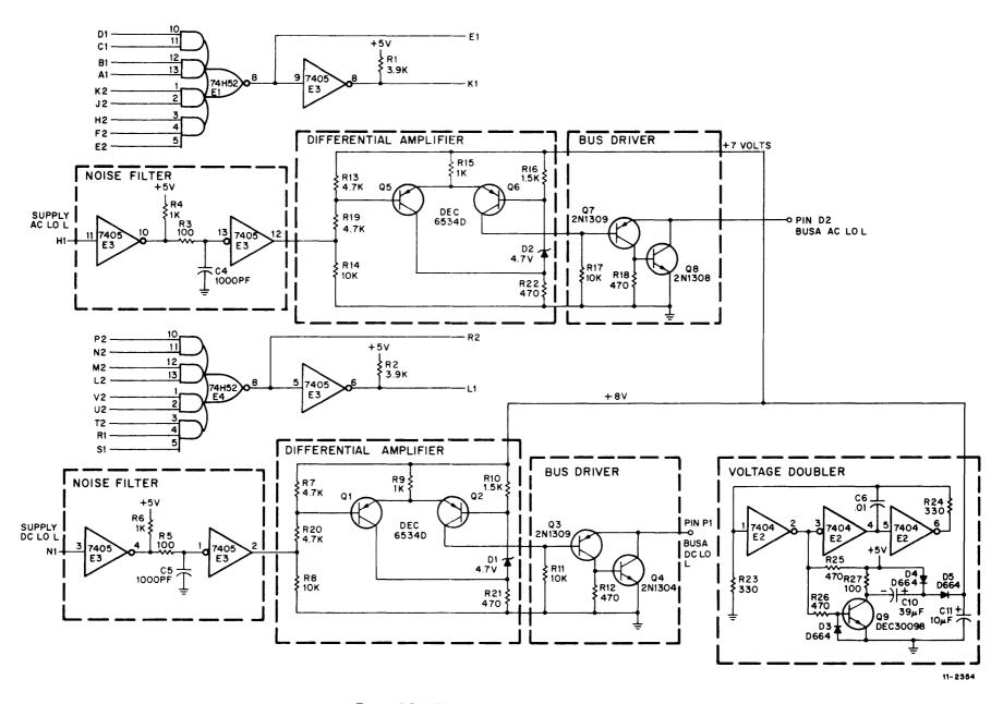
Figure 6-5 UNIBUS Power Fail Drivers Schematic
