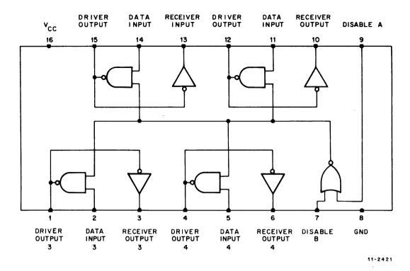
Figure 6-12 M8838 UNIBUS Transceiver Pin Connection Diagram
