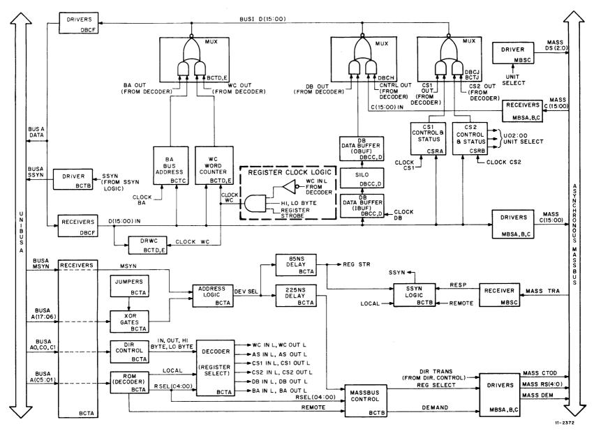
Figure 5-1 Register Control Path
