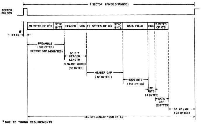
NOTES: 1) WITH SECTOR TYPE FORMAT, NO ADDRESS MARK RECORDING IS NECESSARY.
