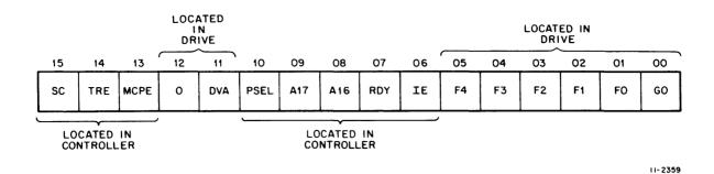
Figure 4-1 Control (RPCS1) Register (776700) Bit Usage
