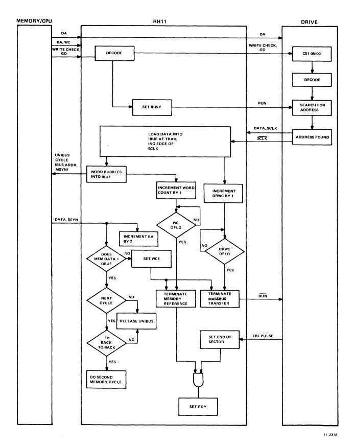
Figure 5-7 Write Check Cycle Interface Diagram
