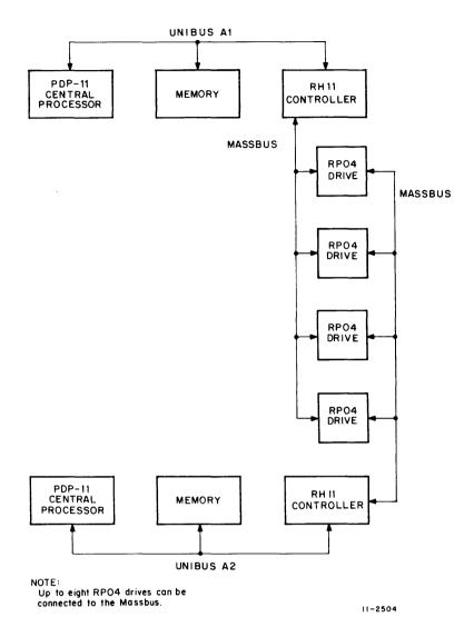
Figure 1-5 Dual Controller Option (With Dual Processor)
