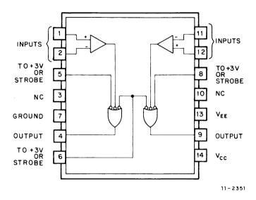
Figure 6-11 75107B Differential Receiver Pin Connection
