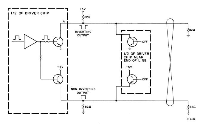
Figure 6-8 Driver Chip Simplified Schematic
