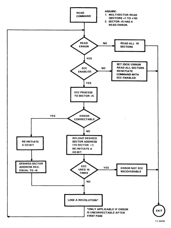
Figure 3-10 Uncorrectable Error Flow Chart Example
