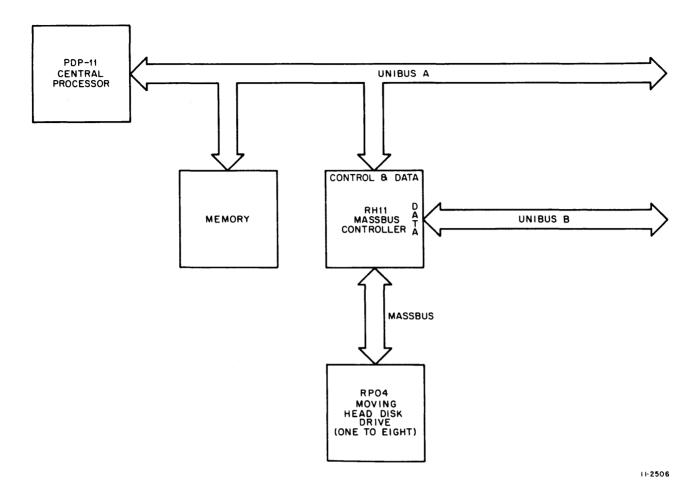
Figure 1-1 RH11 Simplified System Diagram
