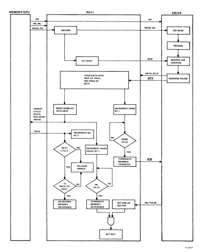
Figure 5-6 Read Cycle Interface Diagram
