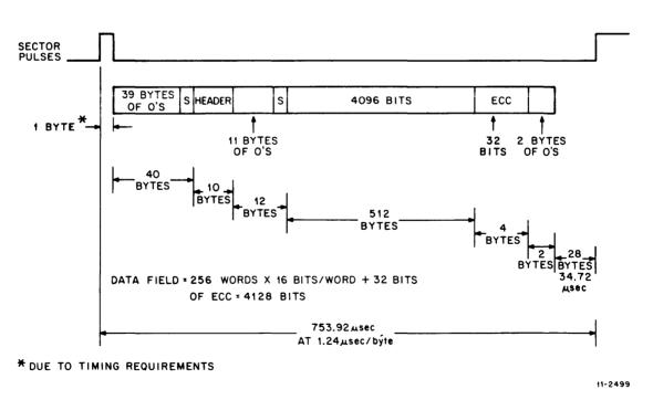
Figure 3-4 Sector Timing (16-Bit Mode)
