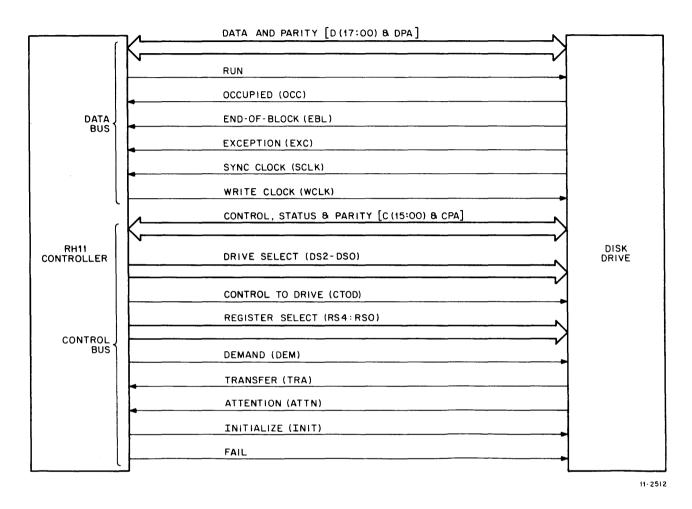
Figure 2-1 Massbus Interface Lines
