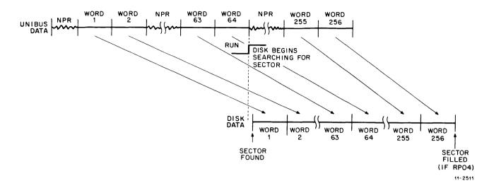
Figure 1-8 Write Data Transfer Sequence
