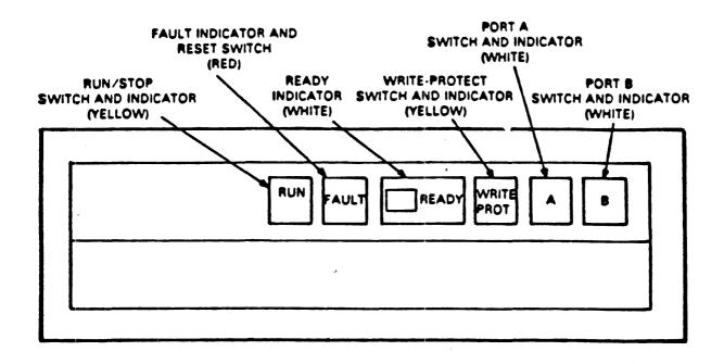
Figure 1 Front-Panel Controls and Indicators
