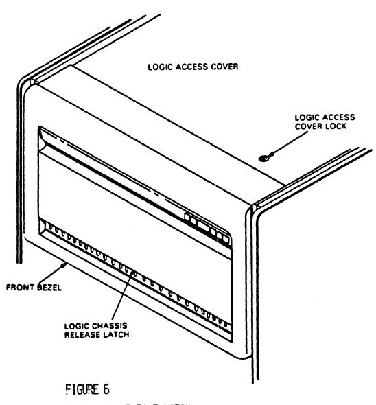
LOGIC CHASSIS RELEASE LATCH
