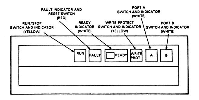
Figure 1 Front-Panel Controls and Indicators
