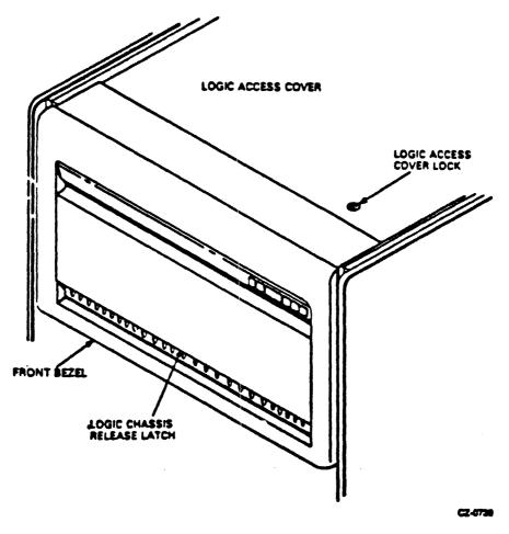
Figure 3 Access to the Inside of the Drive
