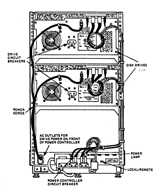
Figure 2 BACK OF AN RA81 DRIVE
