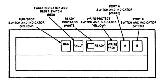
Figure 1 Front-Panel Controls and Indicators
