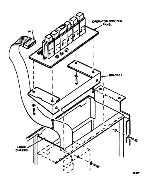
OPERATOR CONTROL PANEL REMOVAL FIGURE 11
