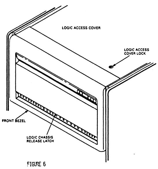
LOGIC CHASSIS RELEASE LATCH
