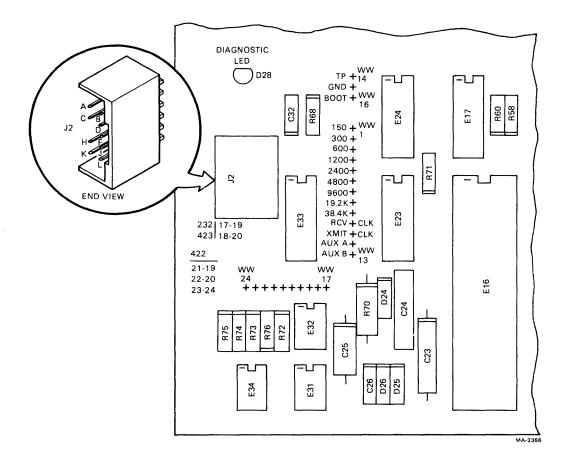
Figure 4-8 Interface Selection Jumper Pin Locations
