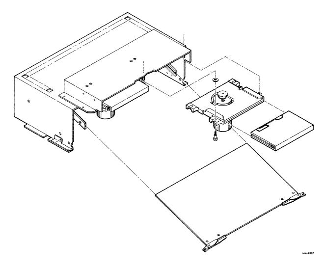
Figure 4-4 Module Removed from Chassis
