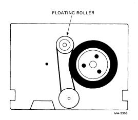
Figure 2-10 Stretch the Belt with the Floating Roller
