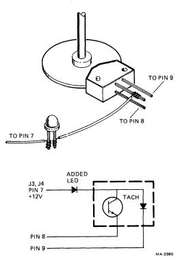
Figure 5-1 Installation of Run Indicator
