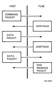
Figure 1-2 An Exchange in Radial Serial Protocol
