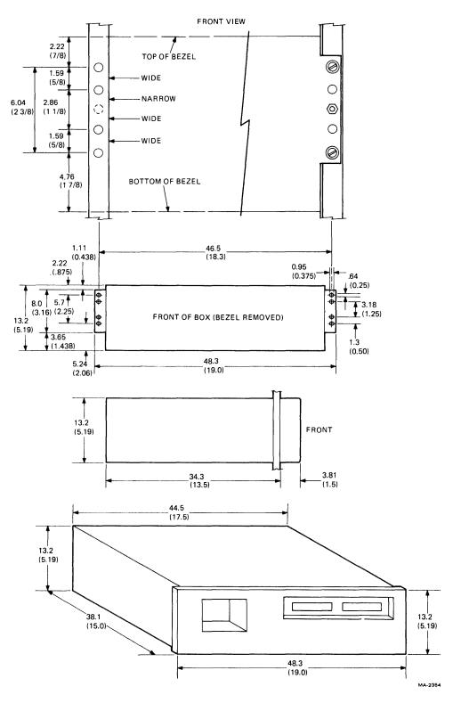
Figure 4-2 Rack Mounting the TU58-CA
