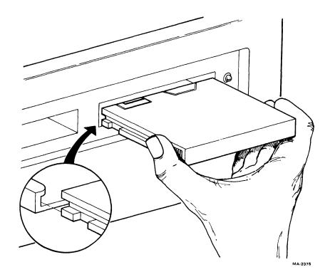
Figure 2-2 Loading a Cartridge
