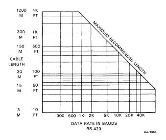
Figure 4-7 Data Rate and Cable Length for RS-423
