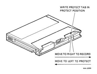
Figure 2-3 Write Protect Tab
