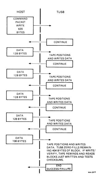
Figure 3-2 Write Command Packet Exchange
