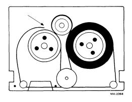
Figure 2-11 Threading the Plastic-Base Cartridge
