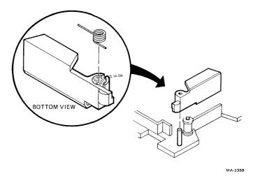
Figure 2-7 Head Gate and Spring
