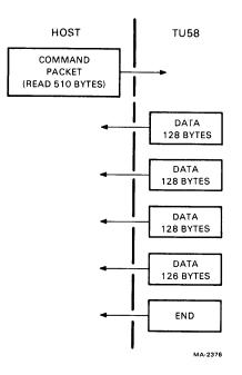
Figure 3-1 Read Command Packet Exchange
