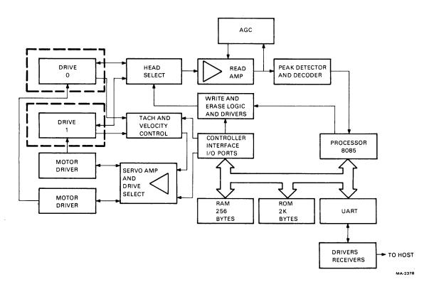
Figure 1-3 TU58 Block Diagram
