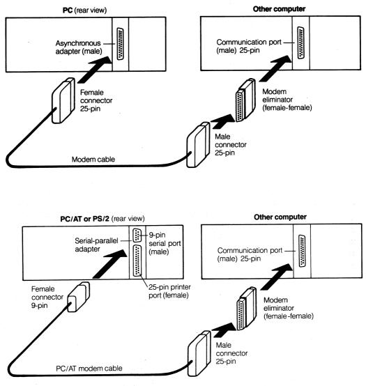
Figure 4-8 Direct Connection, Computer to Computer
