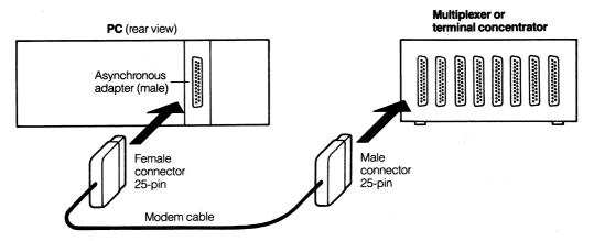
Figure 4-6 Connection to a Multiplexer or Terminal Server
