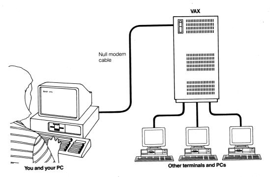
Figure 5-2 Testing the PC-to-Host Connection
