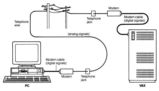
Figure 4-2 Computers Connected by Telephone
