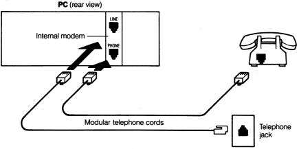
Figure 4-7 Internal Modem Connection
