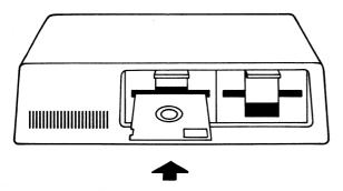
Figure 2-2 Installing Kermit in a Dual Diskette PC
