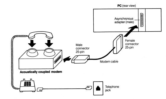
Figure 4-4 An Acoustically Coupled Modem Connection
