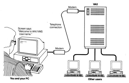
Figure 5-3 Testing a Modem Connection
