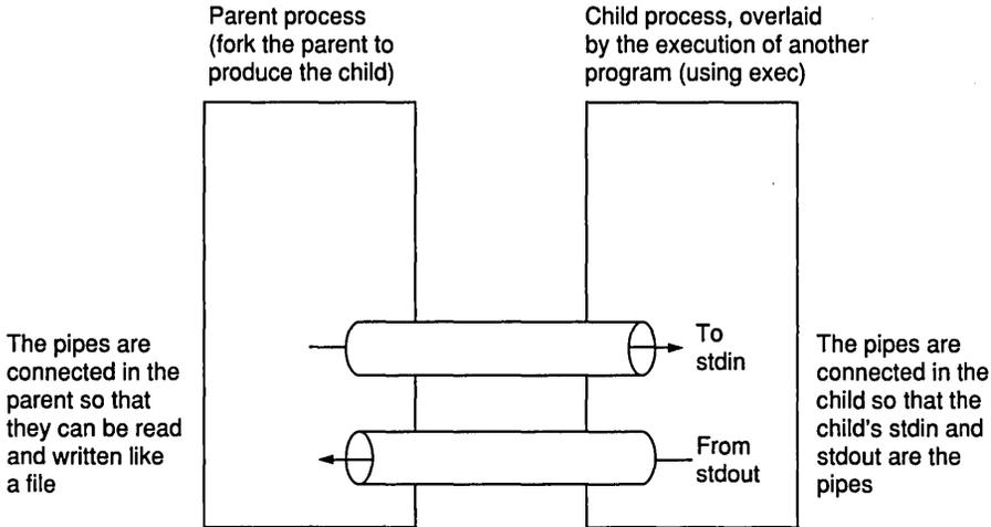
UNIX lets a program split itself into two separately executing copies using the **fork** function. The traditional method for communicating between the two copies is called a *pipe*. The **exec** function lets a program overlay itself with another. A Motif program can thus use the **fork** function to split itself, then overlay its child with a text program using **exec**. The two programs then communicate using pipes. The process is shown in the figure.
