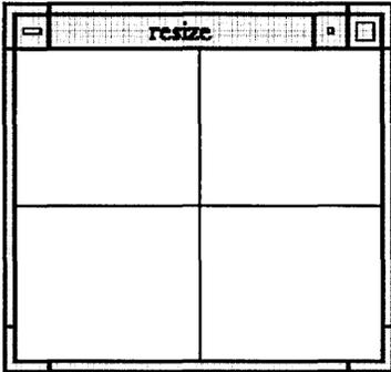
tion handles the redrawing. The `True` value in the `XClearArea` call handles shrinking windows. This parameter generates exposure events after each clear operation.
