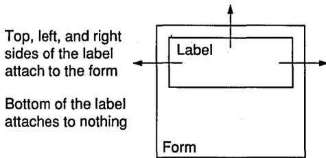
Here the left, top, and right sides of the label are attached to the form. As the form's sides move in response to resizing commands, the attached sides of the label move also, and the label changes width to accommodate the form's size. Since the bottom of the label attaches to nothing, the height of the label does not change, but retains its default height as determined by the label's string and its attributes.
