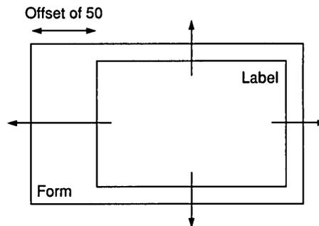
All four sides of the label attach to the form. The label's `leftOffset` resource is set to 50, so its left side remains 50 pixels away from the side of the form to which it is attached. You can create interesting and useful spacing effects using negative offset values as well.
