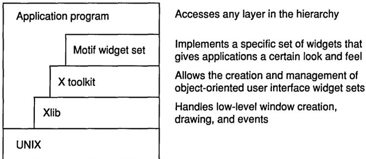
One of the most interesting features of X is its handling of networks. Its fundamental design assumes the existence of networks, so using X over a network is completely transparent. The desire for this transparency drove many of the design decisions that led to X's structure and functionality.
