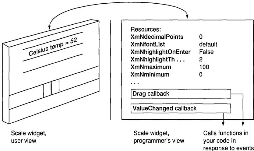
A widget is a user interface object that the user sees in one form—as a picture on-screen—and the programmer sees in another—as a set of resources and callbacks. The figure shows this dichotomy using a scale widget as an example.
