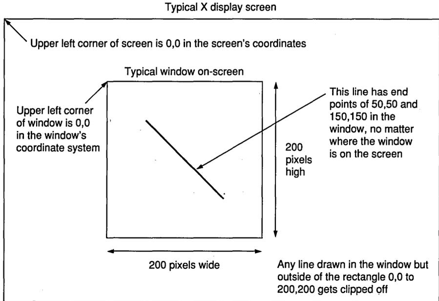
The upper left corner of the window is still  $(0,0)$  no matter where the window appears on the screen.
