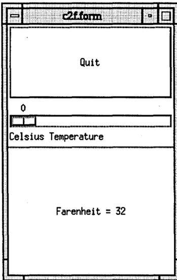
the form widget. Once you create a child of a form widget, the child widget picks up the constraint resource list of the form widget and adds it to its own list of resources.
