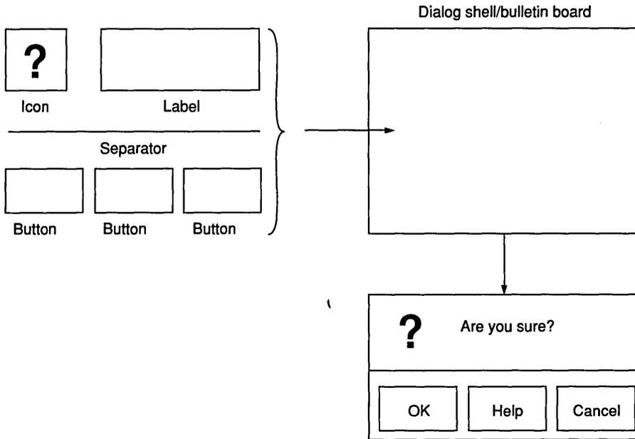
Dialog boxes are composed of a number of separate children bonded into a single widget. The children of a typical message dialog box are shown in the figure above.
