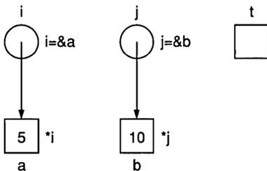
Suppose you accidentally forget the **&** when the **swap** function is called, and that the **swap** line accidentally reads **swap(a,b);**. This causes a segmentation fault. When you leave out the **&**, the value of **a** is passed instead of its address. Therefore, **i** points to an invalid location in memory and the system crashes when **\*i** is used.
