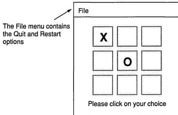
In the process of designing the tic-tac-toe interface, you might get out a piece of scratch paper and sketch out what the interface will look like. Figure 8.1 shows a drawing of one possibility. In larger applications, rough sketches like this can give you a good feel for user interface options quickly.
