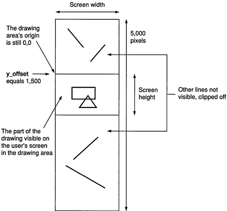
uses a `y_offset` variable and the natural clipping capabilities of a drawing area widget (see Figure 17.13).
