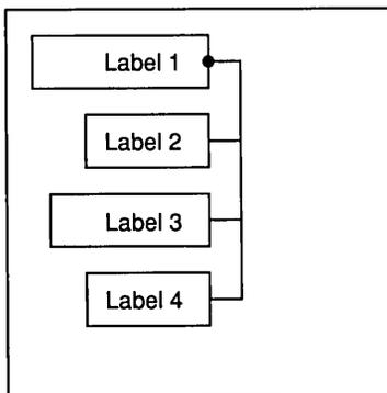
Label 1's right side is attached to the horizontal midpoint of the form. Labels 2, 3, and 4 attach their right sides, using the `XmATTACH_OPPOSITE_WIDGET` attachment, to label 1. As the right side of label 1 moves, the right sides of the other
