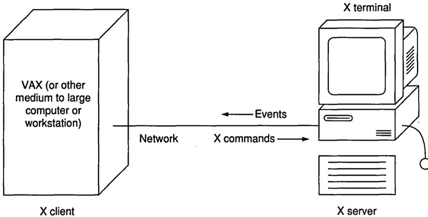
The X Window System provides a basic event-driven programming environment that runs on a workstation or on an X terminal. X controls the mouse, the keyboard, and the screen. Its job is to accept keyboard and mouse events from the user and also to allow applications to create windows on the screen and draw in them.
