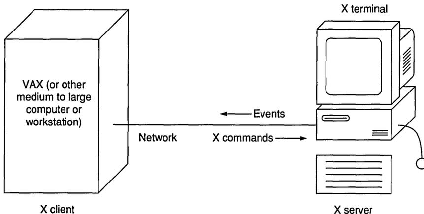
Together, the X terminal's screen, keyboard, and mouse are called a *display*. In order for an X client to do anything on the X terminal, it must use a function to open a communication path to a display. In a pure server/client situation, where the server is an X terminal and the client is running on another computer, the communication path is the network.
