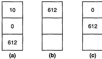
The final line calls the procedure. The numbers preceding the call are the arguments `drawHorizontalLine` requires. The first number is the width, the second is `x`, and the third is `y`. First, 612 is pushed onto the stack, then 0 (`x`) and 10 (`y`).
