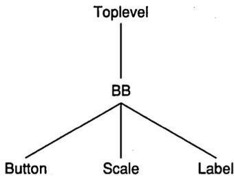
**Figure 5.3 A Bulletin Board Widget Used for the Celsius-to-Fahrenheit Conversion Program**
