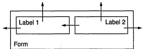
Label 1's left and top sides attach to the form, and its bottom and right sides attach to nothing. The label defaults to its natural width and height. The top and right sides of label 2 attach to the form, the
