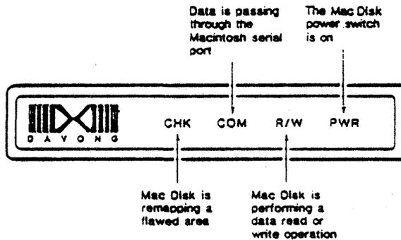
As indicated in Figure 3-1, the indicator lights keep you informed of the operating status of Mac Disk. A complete description of indicator light functions is included in Appendix B.
