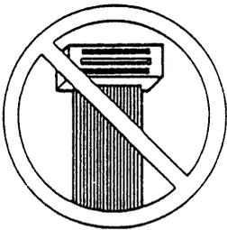
**Using an unshielded interface cable violates FCC-Class B requirements and voids the warranty.**
