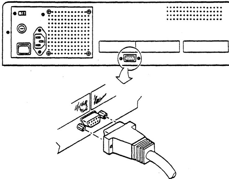
4. With a screwdriver, tighten the screws on the two connectors evenly.
