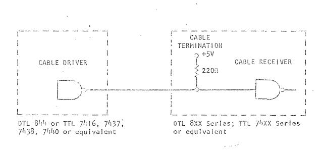
Figure 1-3. Interface Circuits
