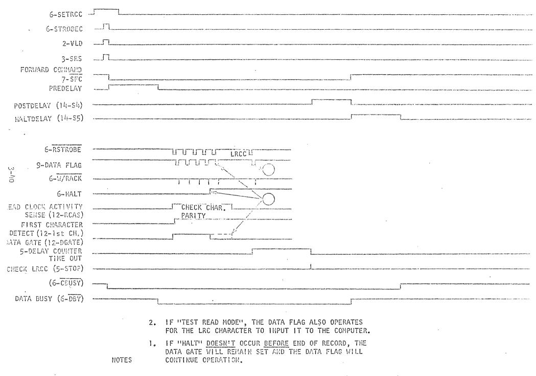
Figure 3.5.9. Read One Record Timing Diagram (7-Track Mode)
