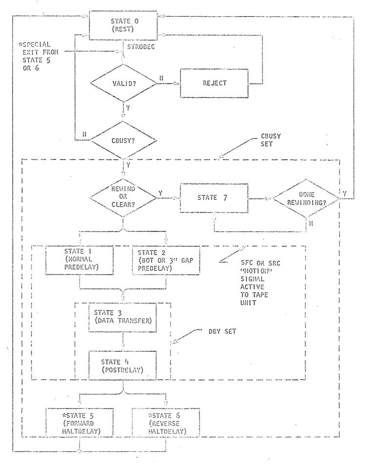
Figure 3-2, Simplified State Flow
