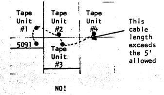
The standard multiple-tape-unit "daisy-chain" configuration requires termination resistors to be deleted from <u>all but the last</u> tape unit. Therefore, the power to the last tape unit must be switched to "ON" when any tape unit is in use. This supplies power to the terminator.
