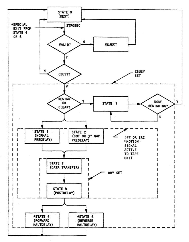
Figure 3-2. Simplified State Flow
