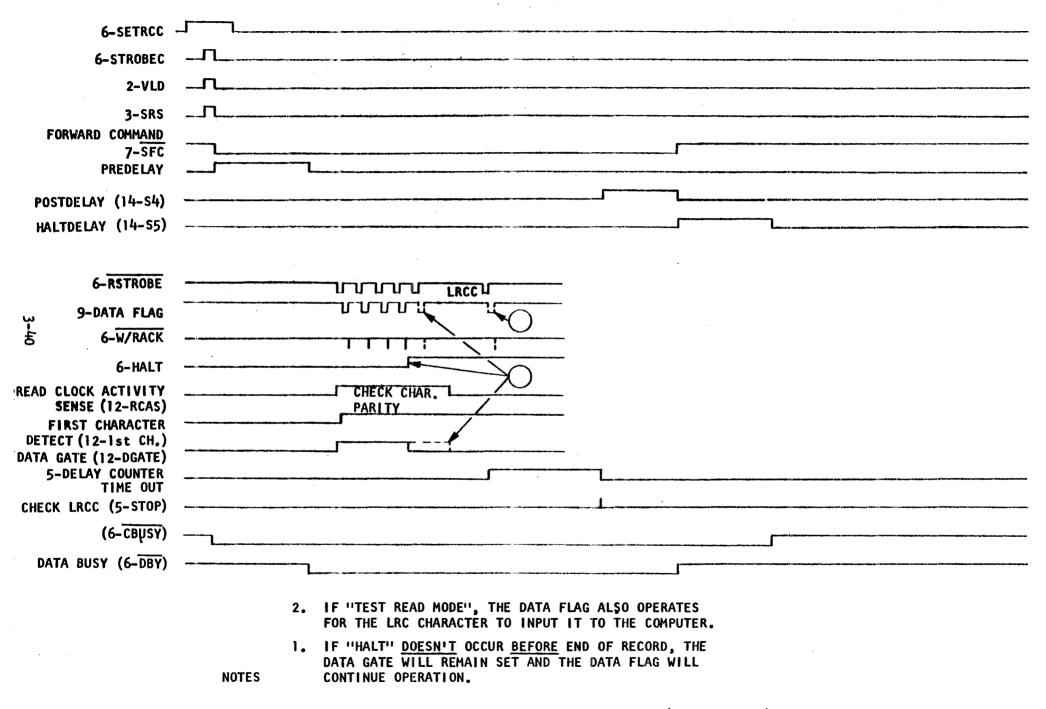
Figure 3.5.9. Read One Record Timing Diagram (7-Track Mode)
