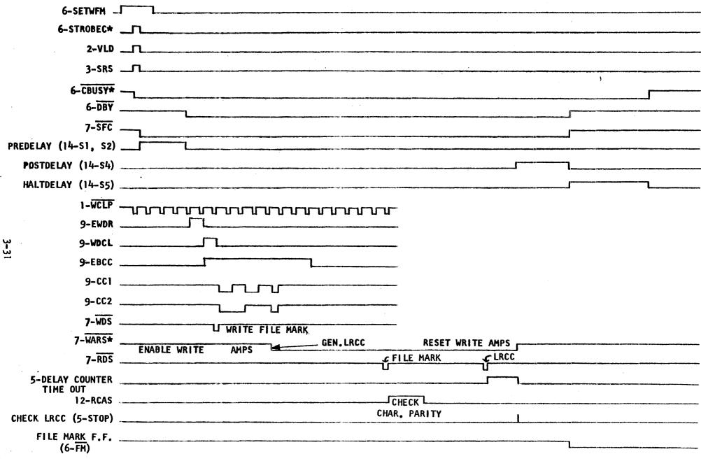
Figure 3.5.3. Write File Mark Timing Diagram (7-Track Mode)
