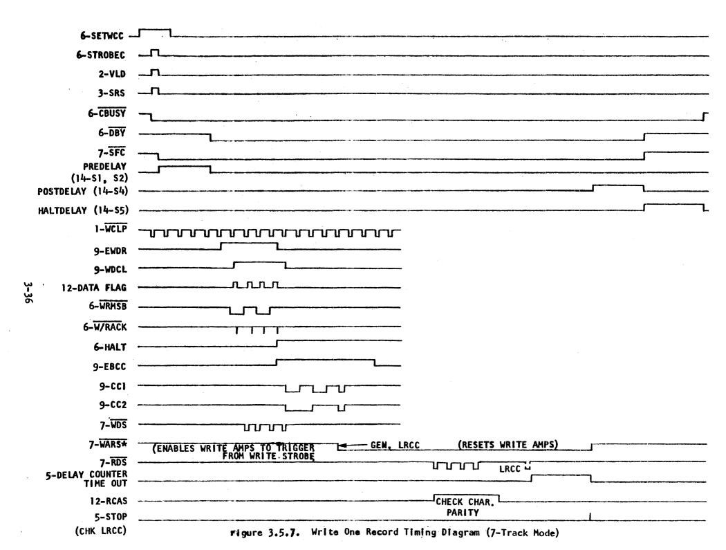
the write current is on for this period. The write data clock flip-flop (9-WDCL) is clocked set one clock time after the 9-EDWR flip-flop to enable write strobes to be generated to the tape unit.
