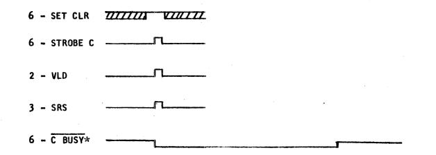
Figure 3.5.1. "Clear" Timing Diagram
