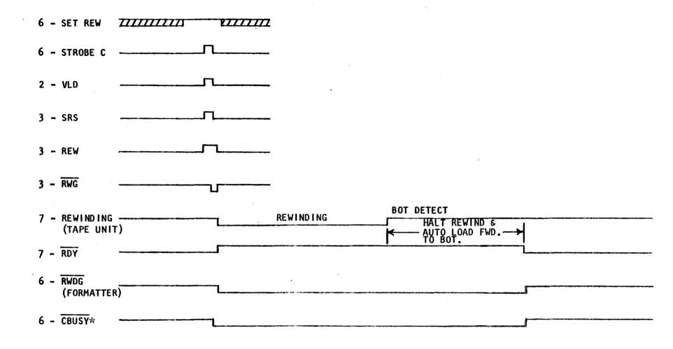
Figure 3.5.2. Rewind Timing Diagram
