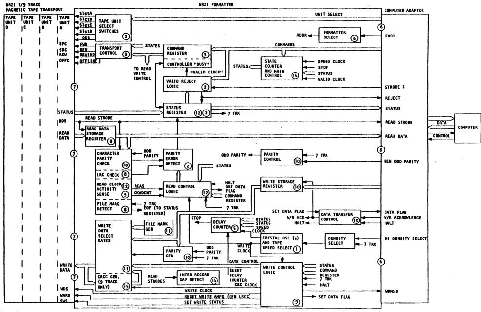
Figure 3-1. NRZI Formatter Block Diagram 3-2
