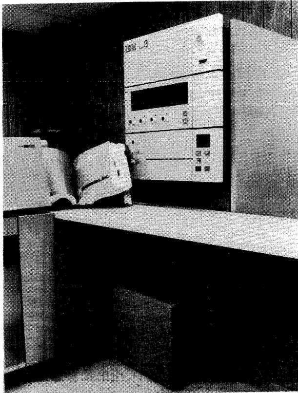
The small box at bottom center holds up to 56K bytes of CFI S/3 semiconductor memory and fits beneath the System/3 operator console.
