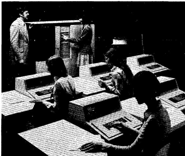
*This 1200 KDS configuration includes five CRT keystations, a chain printer, and the 1204 Control Unit (left rear), which houses a processor, disk drive, tape drive, and control panel.*
