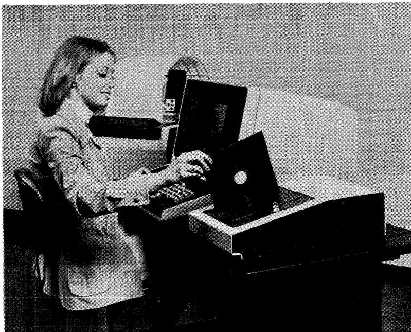
*This stand-alone Sycor 250 terminal consists of a CRT display, keyboard, printer, and dual diskette unit (foreground), a recent addition to the product line. In cluster configurations, a Sycor 250 System can include any mix of up to 32 keyboard/display units and printers.*
