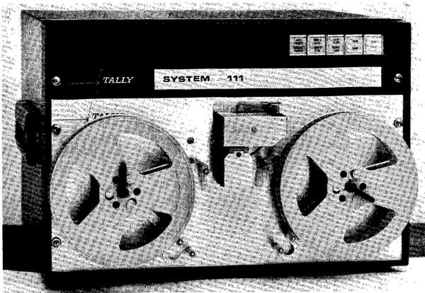
*The Tally System 111 transmits data from punched tape at 120 characters per second and includes reel handling facilities.*
