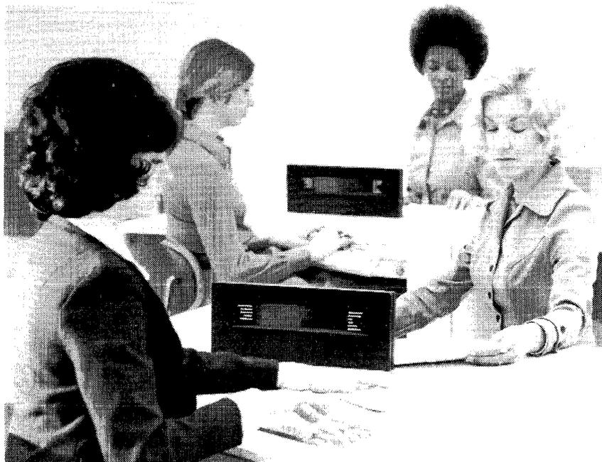
*The 3760 Dual Key Entry Station consists of a desk that houses two keypunch-style keyboards and back-to-back gas-panel display units. A maximum of twelve 3760's can be used in a 3790/3760 Data Entry Configuration to accommodate up to 24 operators.*
