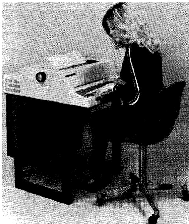
The IS/5741 is a recent addition to the GTE (formerly Novar) family of typewriter terminals. This model includes the Diablo HyType printer mechanism, which features full-character impact printing in both upper and lower case at 30 characters per second. An integral acoustic coupler or wired modem can be added.
