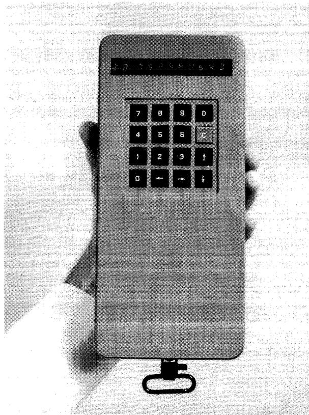
For those of you who remember when the Digitronics Port-A-Verter was the only portable terminal, this self-contained Infopac I from AzurData may seem more like a watch fob. It stores data in a semiconductor memory and transmits it to a central pooling station via an acoustic coupler unit.
