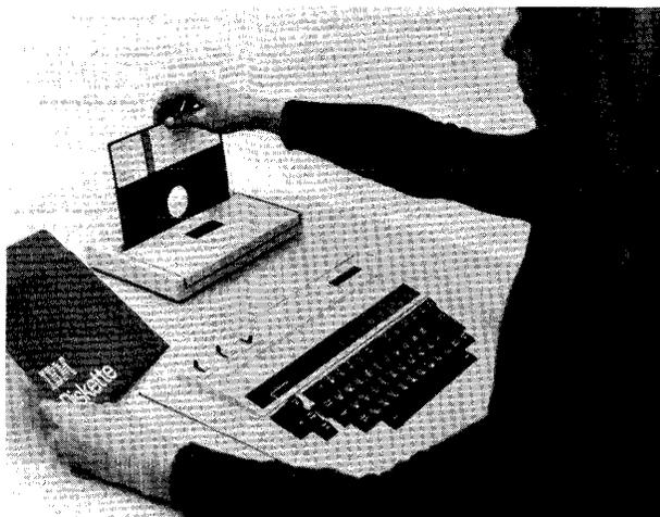
*Inserting a diskette into a 3741 or 3742 Data Station is as easy as inserting a tape cassette or 8-track cartridge into your stereo system. The operator is holding the protective cardboard sleeve in her left hand. The diskette itself is a mylar disk coated on one side with a magnetic material and permanently encased in an eight-inch-square plastic envelope.*
