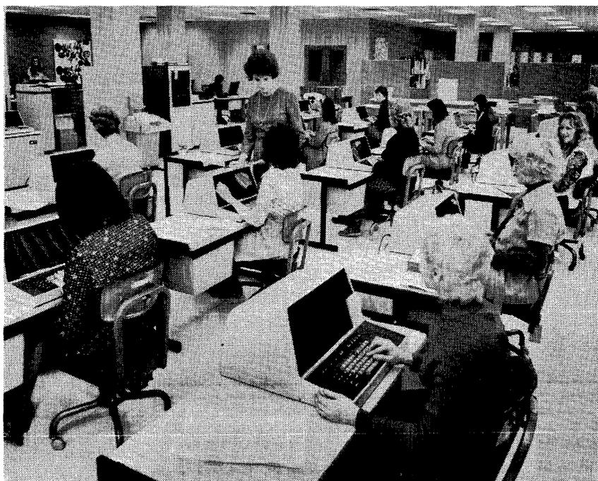
*The powerful Key-Edit 1000 system can accommodate as many as 56 of the CRT keystations shown here. The system's central components can be seen in the background at left.*
