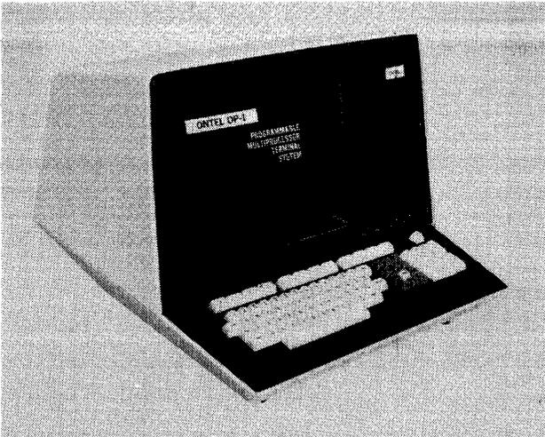
New from Ontel, the user-programmable OP-1 is microprocessor-based and includes up to 16K bytes of memory and a 1920-character screen. The terminal is available with 3M single or dual cartridge tape drives, Diablo 20 or 30 series cartridge disk drives, and an impact printer.
