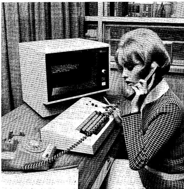
The IBM 2265 is a single-station video display system with optional printer, designed as a remote terminal for IBM System/360 and 370 computers. A maximum of 16 units can be attached to a communications line to operate in a party-line environment.
