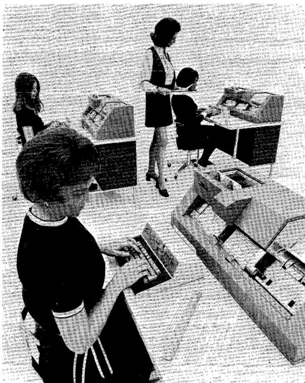
IBM's 129 Card Data Recorder combines the features of vintage card keypunches and verifiers with buffering and some useful new features. The 129 provides punched card installations with most of the capabilities of stand-alone key-to-tape devices without necessitating a switch to another input medium.
