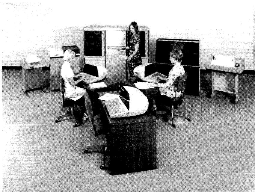
*Shown here are most of the hardware components of the GCS 2100 Data Entry System, including three of the CRT keystations that serve as the principal input units.*
