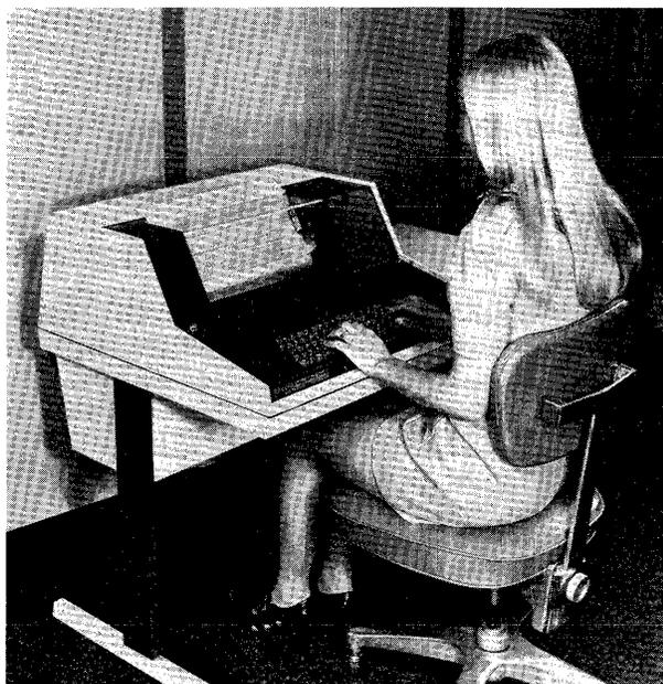
The Execuport 1200 is a high-performance teleprinter terminal designed for special printing applications that require formatting and a forms handling capability. Selectable operating speeds range from 10 to 120 characters per second. The use of paper tape or magnetic tape is optional.
