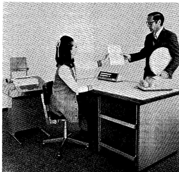
The CMC 5 supervisory console contains a minicomputer, disk drive, and magnetic tape drive. Introduced in May 1971, the CMC 5 system handles up to 16 keystations and provides most of the capabilities of the larger KeyProcessing systems at a considerably lower price.
