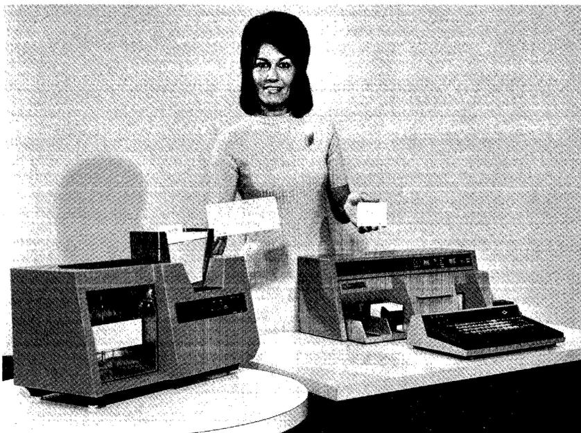
*Feature 1020 equips a Decision Data 9601 or 9610 Data Recorder or 9660 Sorting Data Recorder (Report 70D-363-02) to perform 80-column to 96-column card conversions by adding an 80-column card reader (at left). Card files are converted at a speed of 60 to 120 cards/minute.*
