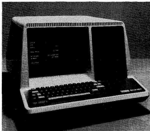
Digital Equipment's attractive VT50 DECscope, introduced in September 1974, features a 960-character screen with typewriter-style keyboard and an integral non-impact hard-copy device (not visible). Its low price of \$1,250 (in unit quantities) makes it a formidable competitor for the Teletype replacement market.
