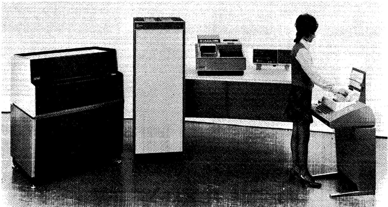
*A basic HASP terminal configuration of the Westinghouse 2550 Satellite Processor. Components shown include a processor with 8K 16-bit words of memory, a medium-speed card reader and line printer, and a Teletype ASR 33 used as a console.*
