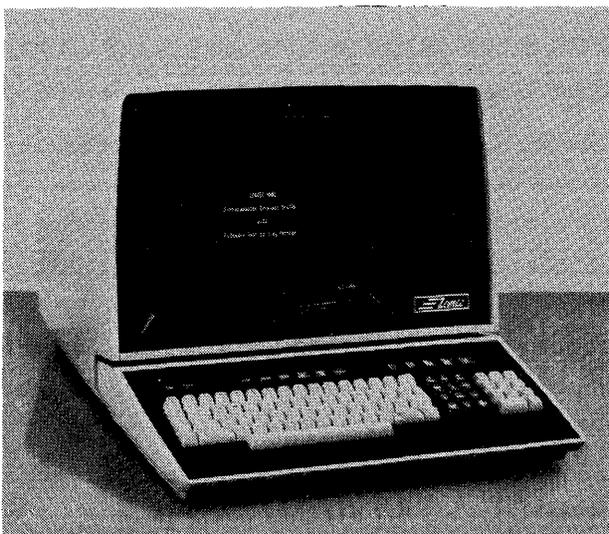
The Zentec 9002 is one of a new breed of terminals by relative newcomers to the display terminal market. This user-programmable terminal features microprocessor control, up to 16K bytes of memory (including ROM, PROM, and RAM), a 1920-character screen, and a detachable keyboard.
