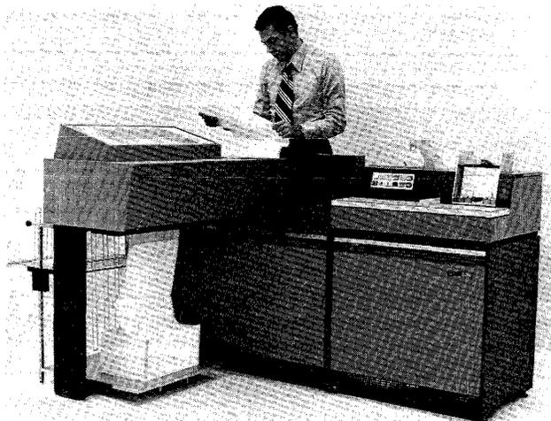
The 3780 consists of a 425-lpm bar printer (left), control unit (center), and 600-cpm card reader (right). It offers transmission speeds of up to 7200 bits per second.
