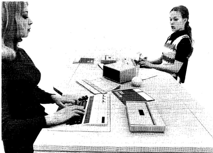
*The IBM 3740 Data Entry System records data on a diskette instead of on cards. One diskette holds the equivalent of a full box of cards, but the diskette is only eight inches square and a fraction of an inch thick. Shown above is the 3742 Dual Data Entry Station, which accommodates two operators at the same desk. Each operator records data on a separate diskette.*
