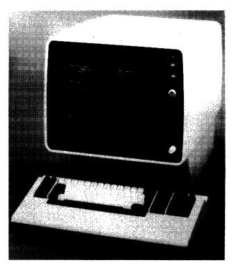
Telex has added SDLC capability to the 276 Control Unit Display Station. The 276 offers control of up to eight devices, and is functionally compatible with the IBM 3276.
