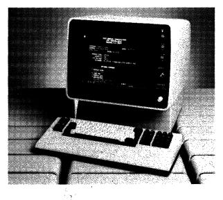
The 279 Color Display Station is functionally compatible with IBM's 3279 Model 2A. The 279 features four-color capability—red, white, blue, and green.
