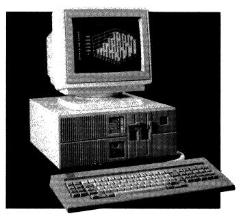
The Telex 1280 Intelligent Workstation offers high-speed, 16bit processing with optional on-line 3270 communications support. The 80286 microprocessor, 512k bytes standard internal memory, and the MS-DOS 3.1 operating system contribute to the 1280's performance.
