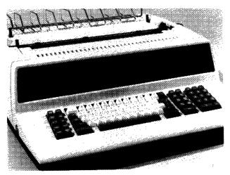
The Telex 767 Keyboard/Printer Terminal is equipped with a console panel which includes LED indicators, a 3-digit display, and a touch pad. Model 2, pictured here, provides a metalized printwheel mechanism for letter quality printing.
