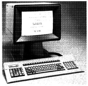
TEC's ET80 display terminal features a 15-inch screen, positive display format, and a low-profile keyboard. The CRT unit is pedestal-mounted, and can be adjusted horizontally and vertically. All TEC terminals feature a display capacity of 2000 characters, arranged in 25 lines of 80 characters each.
