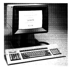
TEC's ET80 display terminal is designed to meet international ergonomic requirements for video display terminals. The ET80 includes a 15-inch adjustable display monitor with a positive dark-on-light display, and a low-profile keyboard that conforms to the DIN standards for ergonomics.
