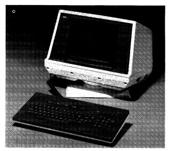
The 7900 Model 1, introduced by NCR in 1979, has been ergonomically redesigned. Standard features now include a 12-inch amber display screen, tilt/swivel base, and a detachable keyboard.
