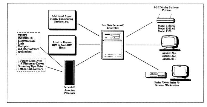
Figure 1. The Series 610 Associate Processor provides local processing for up to 32 Lee Data terminal, printer, or workstation users. Older Lee Data equipment, like the Series 700 Personal Workstation, is also supported.
