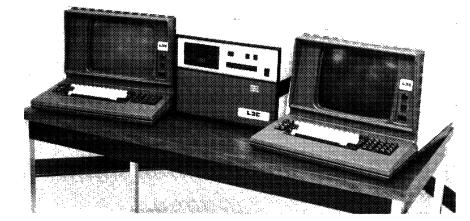
Lee Data Corporation's Model 310 Remote Control Unit is shown here flanked by two of the company's All-In-One SOFTPRINT Display Stations. The Model 310 Remote Display System allows for remote clusters of devices (up to 32, including any mix of display stations and printers). The system emulates the operating characteristics and features of the IBM 3270 Information Display System.
