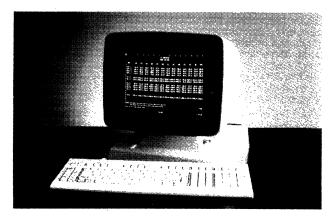
Lee Data's new Model 1214 Display Terminal is available in four models, including All–In–One versions which provide four selectable display formats. The terminals include a 14-inch screen, low-profile keyboard, and a compact enclosure with a reduced footprint.
