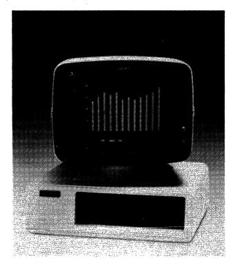
The Series 70 Personal Workstation emulates the IBM 3270-PC. Like the 3270-PC, the Series 70 provides windowing capabilities, enabling the user to run seven concurrent sessions (four interactive host sessions, a personal computer session, and two note pads). The unit can display up to 16 colors in PC graphics mode, or up to 8 colors in host graphics mode.
