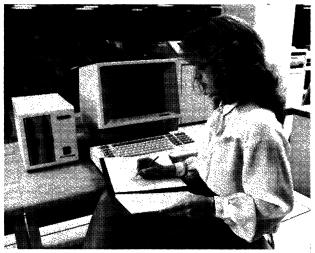
Users of the Harris 9200 Information Processing System can now add personal computing capabilities to the system as an option. Harris' Integrated Personal Computing option consists of a multi-functional terminal with 64K bytes of memory, two 8inch, 1MB diskette drives, and the CP/M operating system.
