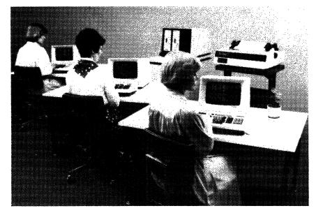
The 8180 Interactive Terminal System pictured above operates in IBM 3270 emulation mode while concurrently performing such enhanced functions as queued transaction handling, spooled printing, and local format storage.
