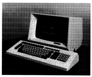
The Harris 8180 System offers IBM 3270 emulation. The display offers screen capacities from 480 to 1920 characters, on a 12-inch (diagonal) screen. The keyboard is detachable.
