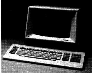
The Harris 9178 Display Terminal can be configured with both the 9100 and 9200 Information Processing Systems. The 9178 features a 12-inch display screen with amber or green phosphor characters, and a 109-key, low-profile keyboard.
