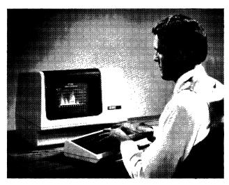
DEC's VT125 features business graphics, as well as alphanumeric, capabilities. Using DEC's Remote Graphics Instruction Set (ReGIS), pictorial data is created and stored as simple ASCII text. An upgrade kit is available to enable a standard VT100 to be configured with the graphics capabilities of the VT125.
