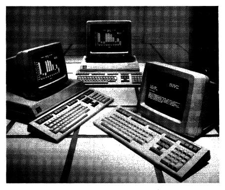
The Digital VT200 family of video display terminals consists of three models. The VT220 features full VT100 compatibility, the VT240 provides bit-mapped graphics architecture and text/graphics capabilities, and the VT241 replaces the monochrome display of the VT240 with a color monitor.
