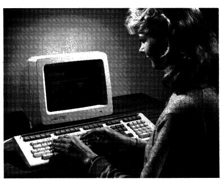
The Digital VT220 boasts full VT100 compatibility, including 80-/132-column display capability and compatibility with the ANSI X3.64 standard. As was the case with the VT100, several vendors have recently introduced terminals designed to emulate the VT220.
