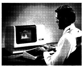
The VT125 features business graphics, as well as alphanumeric, capabilities. Using DEC's Remote Graphics Instruction Set (ReGIS), pictorial data is created and stored as simple ASCII text.
