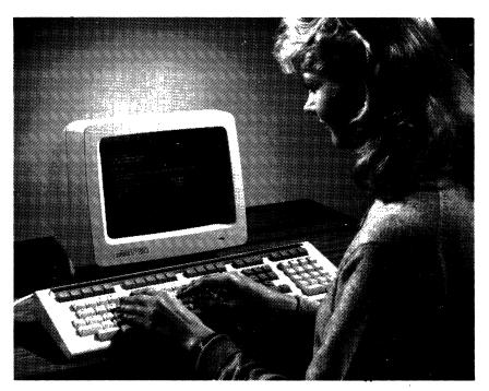
The VT220 is the low-end model in DEC's new VT200 terminal family. The VT220 features two-piece modular construction, with a 12-inch monochrome display and a detachable, low-profile keyboard. As with all of the new VT200 terminals, the VT220 boasts full DEC VT100 compatibility, including 80-/132-column display capability and compatibility with the ANSI X3.64 standard. As was the case with the VT100, several vendors have recently introduced terminals designed to emulate the VT220.
