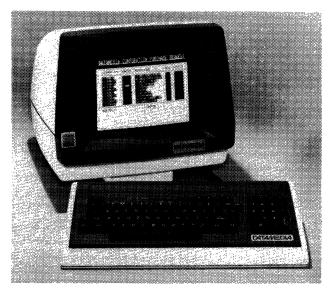
Datamedia's Excel Series of display terminals are ergonomically designed. The display monitor can be tilted from 5° to 15° to achieve the most comfortable viewing angle. The keyboard is detachable, and connected to the monitor via a six-foot coiled cord. A choice of 12-inch or 14-inch screen sizes is available.
