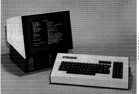
The Elite 1520A has the same attractive physical appearance as the other members of the Elite family and offers many of the features of the top-ofthe-line 2500A, A key feature is its support for both APL and ASCII.
