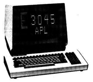
The Datamedia Elite 3045A, a buffered APL/ASCII terminal, features a single-page video memory that displays 1920 alphanumeric characters in a 24-line by 80-column format. As with all of the Elite series terminals, the keyboard is detachable.
