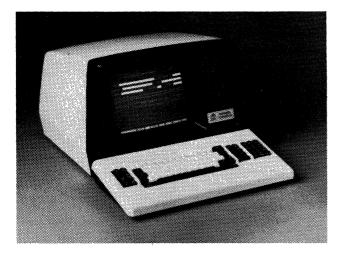
Beehive's new DM5 is a microprocessor-based smart terminal designed to fit entry-level applications, while offering editing capabilities and block, as well as character-by-character, transmission. The DM5A, pictured above, offers all of the features of the basic DM5, plus a numeric pad, program function keys, and an auxiliary printer interface.
