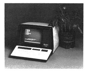
The DM83 is Beehive's Burroughs TD830/MT983 emulator. The DM83 operates in all communications modes (asynchronous, isochronous, synchronous), and supports all major Burroughs polling protocols. The terminal can operate as a standalone unit or as part of a daisy chain cluster.
