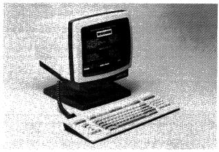
Beehive's newest display terminal is the ATL-004. The second member of the company's ATL series, the ATL-004 features a 14-inch display with tilt/swivel capability, an 80/132-column display format, a detachable, low-profile keyboard which conforms to the DIN standard for ergonomics, and a range of smart terminal features.
