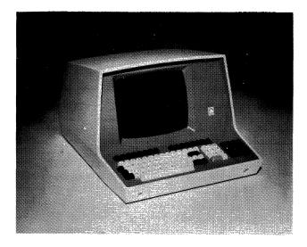
The B 100 shown above was introduced in June 1976 and is the entry-level model in Beehive's family of display terminals. The B 100 is Teletype compatible and features an addressable sensor and a 960- or 1920-character screen.
