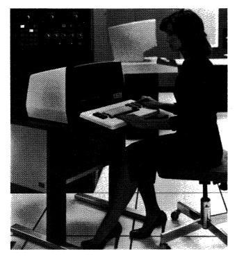
The DM3270 Control Unit Display Station offers "enhanced emulation" of the IBM 3276-2 stand-alone station. The DM3270 can satisfy remote site requirements for both single- and multi-station applications.
