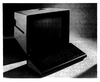
This Model 400E terminal shows the 15-inch "Smart Monitor", detachable keyboard, and compact cabinetry (15 inches wide, 14 inches high, and 13.6 inches deep) used on all Ann Arbor Terminals. Screen capacity shown is 1920 characters; options permit the 400E to display 960 double-wide or 480 double-size characters. Other models support a 3200- or 4800-character screen capacity using the same monitor.
