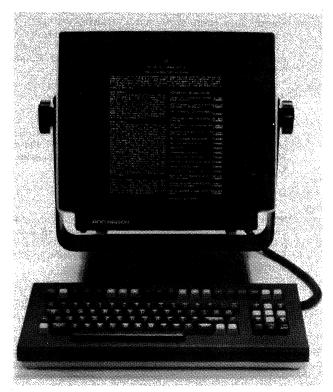
The Guru, Ann Arbor's newest terminal, offers a display format expandable to 66 lines by 170 characters and split screen capabilities. The unit shown above features the "portrait display" screen format and a tilt-and-swivel viewing stand.
