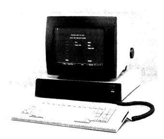
The E4549 is a four-color display terminal available in two models. The E4549-42 provides a 1,920-character display capcity; the E4549-43 provides selectable 1,920- and 2,560-character display capacities. Both models include a 13-inch screen and choice of detachable keyboards.
