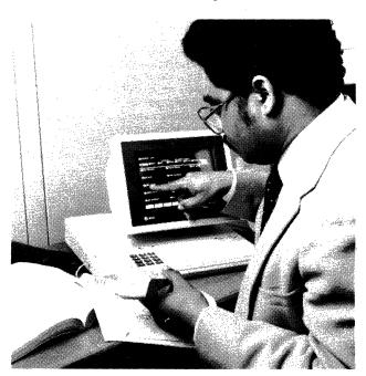
The AT&T Personal Terminal Model 510 is an integrated voice/data terminal (IVDT) equipped with a touch-sensitive screen. Designed for use in conjunction with the AT&T System 75 and System 85 PABXs, the Model 510 provides one-touch access to voice and data functions.
