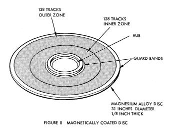
The magnetic material is a finely divided high-coercivity ferrite powder which is bonded together and to the disc by a tough thermosetting plastic. After finishing, each disc is inspected and tested to ensure that it contains no areas which could cause or might lead to "bad spots" in service.
