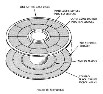
Each sector contains a header as well as a record. In addition, there are gaps before the header, and between the header and the record to accommodate mechanical tolerances, including the physical difference between the erase gap and the read/write gap.
