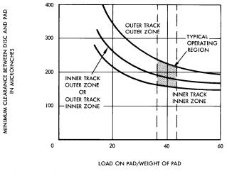
FIGURE IV THE CHARACTERISTICS OF THE HEAD PAD
