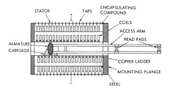
FIGURE V THE DIGITAL POSITIONER
