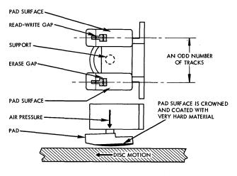
FIGURE III VIEWS OF PAD STRUCTURE
