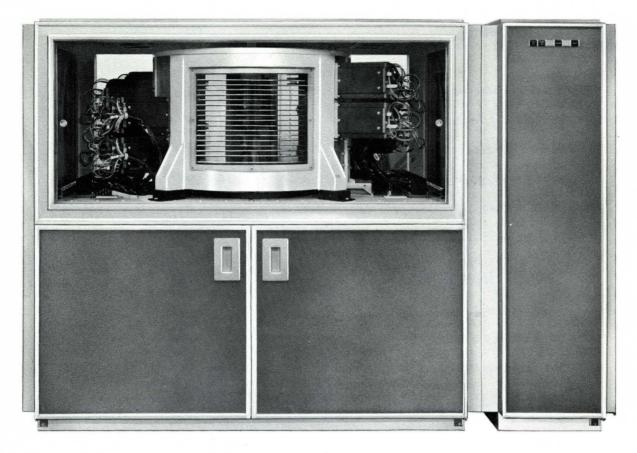
dp/f-5022  ${\tt DISCFILE}$  System consisting of a  ${\tt DISCFILE}$  Unit and Logic Unit
