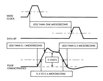
FIGURE XVI CLOCK AND DATA CHARACTERISTICS
