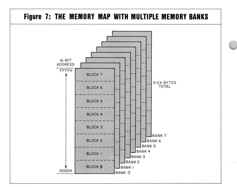
memory bank, and each reset bit (logic 0) disables its bank. Control byte bit 7 (MSB) controls memory bank 7, bit 6 controls memory bank 6, etc.
