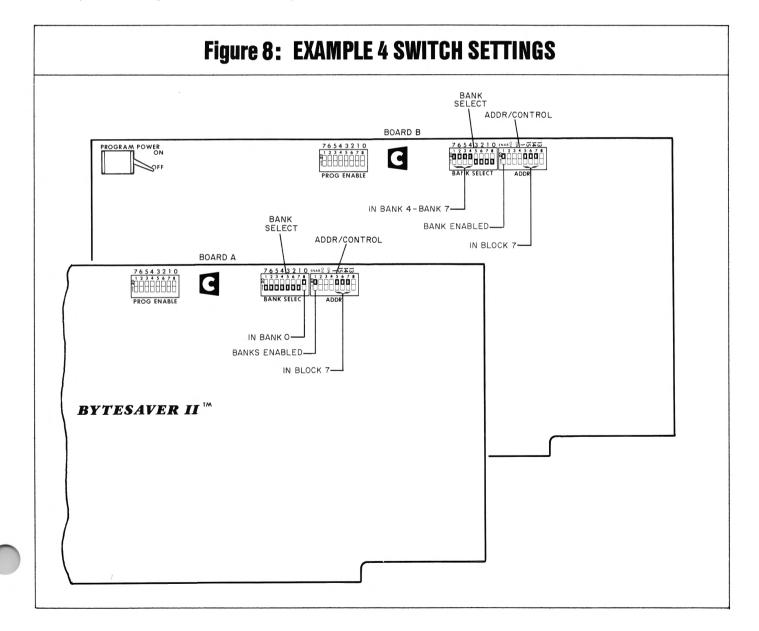
To continue the same sample, the sample programs ahead illustrate how to memory bank enable and disable the two boards.  Executing the instructions below activates memory banks 2 and 3, and de-activates all other memory banks. The instructions then place both board A and board B in inactive memory banks (both boards inaccessible).
