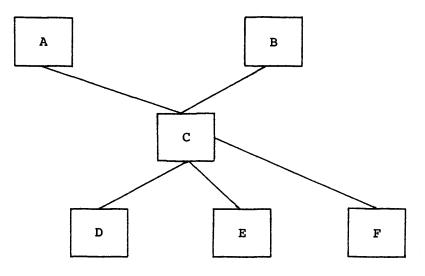
Figure 2-4. Invalid segment tree (multiple root segments)
