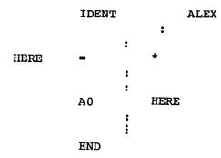
SEGLDR processes the A0 HERE instruction's jkm field as an extended block relocation since HERE is a label local to module ALEX. If the relocation quantity to be added (the base address of module ALEX as assigned by SEGLDR) results in a value exceeding the reserved 22-bit field, SEGLDR issues an error.
