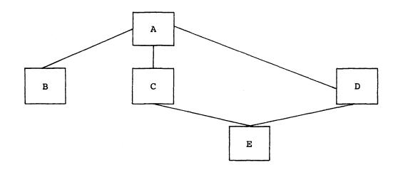
Figure 2-5. Invalid segment tree (multiple immediate predecessor segments)
