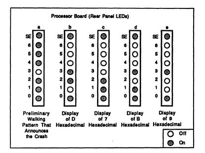
Figure 12–11 Sample Processor LED Crash Code Sequence
