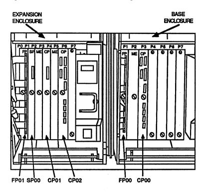
Figure B-3 Processor Board Numbering Scheme
