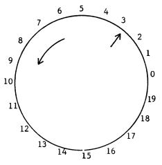
The number 2 is only one unit from the present position but in a reverse direction. Remember that the additive device cannot move in that direction. Instead, it must move 19 units in the forward direction instead of 1 unit in the reverse direction (-1).
