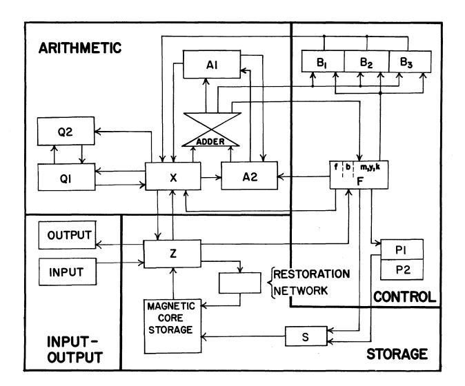
Figure 4-13. Basic Computer Sections
