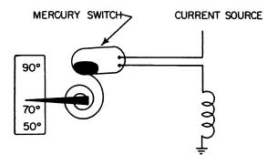
Temperature drops to  $72^{\circ}$  - coiled spring retracts - opens gas value - furnace comes on - temperature rises.
