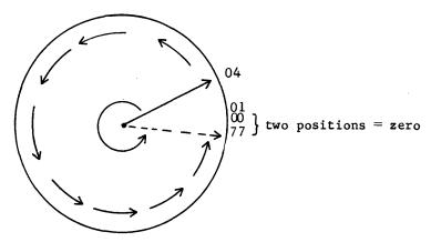
The extra position with a discrete value of zero caused us to count zero twice, which caused the answer to be one less than it should have been.
