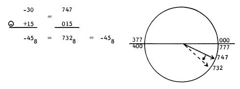
Comparison of the two foregoing examples clearly illustrates what causes overflow. In the first example, the difference between the two operands was -45. The modulus of the device only permits expression of operands between -37 and +37. The second example used the same operands but the modulus of the device permits expression of values between -377 and +377.
