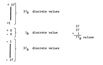
A 6-bit unsigned device could express  $100_8$  discrete values whereas a 6-bit signed device should express 1 less or 77<sub>8</sub> discrete values. Therefore, the modulus of a 6-bit <u>unsigned</u> device would be expressed as  $2^6$  but the modulus of a 6-bit <u>signed</u> device would be expressed as  $2^6$  - 1 ( $2^6 = 100_8$ ,  $2^6$  - 1 = 77<sub>8</sub>). A 24-bit signed device would have a modulus of  $2^{24}$  - 1 and a 24-bit unsigned device would have a modulus of  $2^{24}$ .
