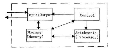
By the previous definitions, it should be apparent that all four sections are necessary to an automatic computer. The dotted lines around the four sections are the outer dimensions of an automatic computer.
