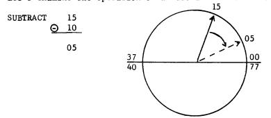
When we passed through zero with an additive device, we always had an EAC; therefore, it seems probable that we should witness some strange phenomena when passing through zero in the reverse direction.
