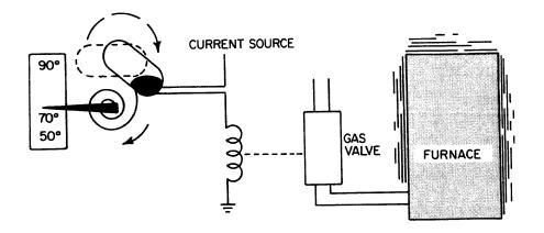
Now you manually readjust thermostat to  $50^{\circ}$  - switch opens - valve closes - furnace goes off.
