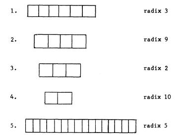
Back to the definition of modulus and how the modulus of a device is expressed: The radix of a number system raised to some exponent.
