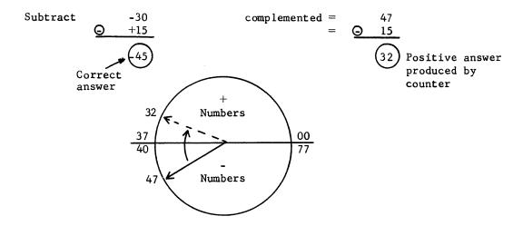
The counter has produced an incorrect result because, again, the modulus of the device has been exceeded. If the same two operands are used but the modulus of the device is expanded to  $8^3$  -1, the answer will now be correct.
