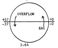
If subtraction is required and the device is additive, the subtrahend is <u>always</u> complemented and addition is performed.
