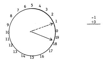
When the device is moved forward 3 positions, as indicated by the number to be added, we find that the arrow now points to the 2 -- again the correct answer. In the first example, we effectively subtracted 1 by adding its complement (19); in the second example, we added 3 to -1 (19).
