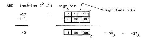
The result indicates the correct answer to be  $40_8$ . However,  $40_8$  expressed in a 6-bit signed device indicates an actual value of  $-37_8$  which is, of course, incorrect. The modulus of this device is  $77_8$  and the range of operands is from -37 to +37.
