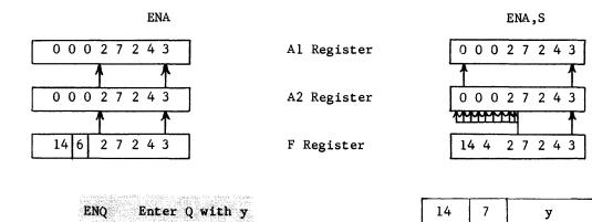
Clear the Q register and enter with the 15-bit operand y. Similar to ENA except that the Q register is involved.
