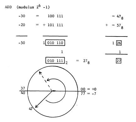
In the first example, we added two positive numbers and the result was negative. In the second, we added two negative numbers and the indicated result was positive. The indicated answer was incorrect because the sum of the numbers in both examples exceeded the modulus of the device and changed the sign bit.
