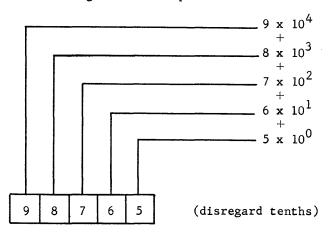
The following odometer reading could be expressed in radix 10 as
