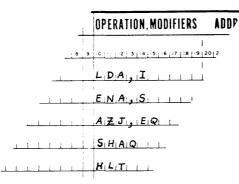
The operation field contains a mnemonic instruction code with related modifiers, a pseudo-mnemonic instruction (to be explained), or the octal values 00-77 to indicate the machine code for an instruction. The field begins in column 10 and is terminated by the first blank. If the address field is blank, the assembler translates it as a 00 machine code.
