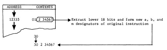
Instruction now indicates that indexing is again required. If (B2) is equal to 66666, M + (B3) = 23456:(34567 + 66666 = 23456). M is now 23456, the address of the operand.
