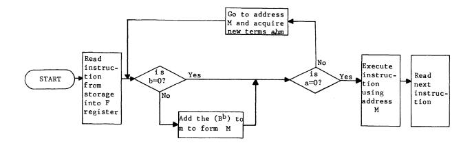
Figure 4-11. Formation of execution address (M)
