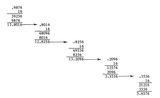
Step 2. Record the results of each operation and convert results to hexadecimal equivalent. The first character obtained becomes the most significant of final answer.
