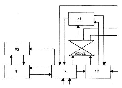
Figure 4-15. Arithmetic Section
