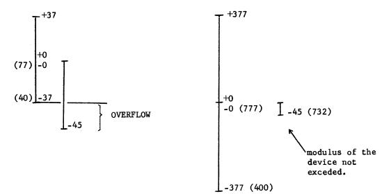
Remember the rule for overflow? If two numbers of unlike signs are subtracted and the result has the same sign as the subtrahend, the modulus of the device has been exceeded and OVERFLOW has occurred.
