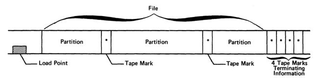
On a labeled S or L tape, an EOFI label replaces the second terminating tape mark. The system recognizes the EOFI label as end-of-information for the tape and initiates end-of-information processing as indicated by the user.
