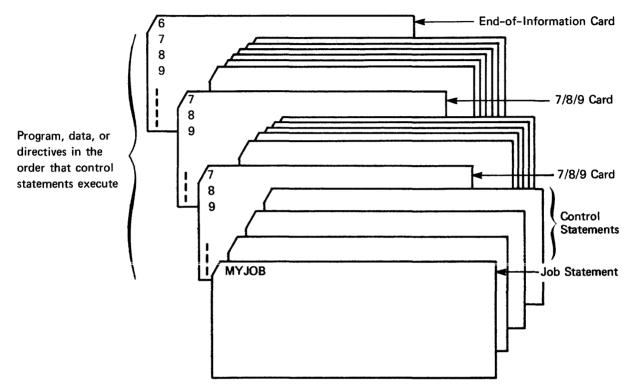
The first card of any deck (figure 2-1) is the job statement; the last card has a 6/7/8/9 multiple-punch in column 1. Cards with a 7/8/9 multiple-punch in column 1 divide the deck into sections.<sup>†</sup>
