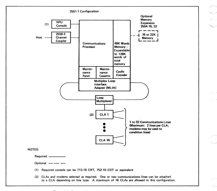
Figure 1-8. Typical NPU and Peripheral Hardware Configuration
