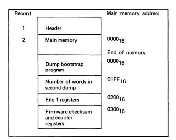
Figure 3-1. Format of an NPU Dump
