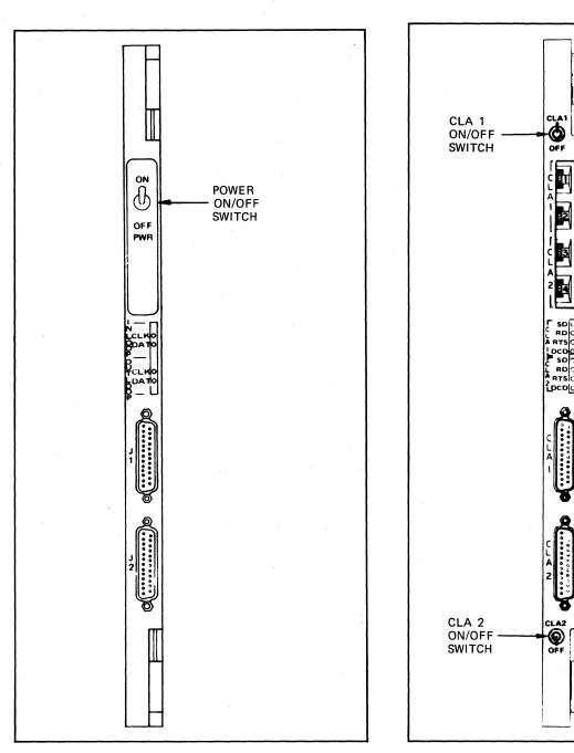
Figure 5-2. CLA Circuit Card ON/OFF Switch Location
