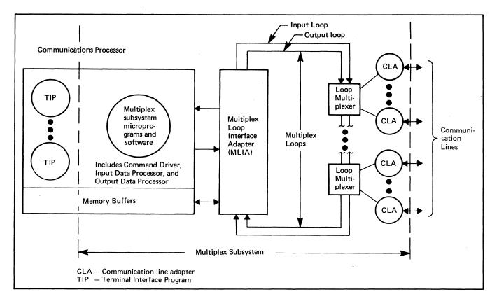
Figure 2-2. Basic Elements of the Multiplex Subsystem
