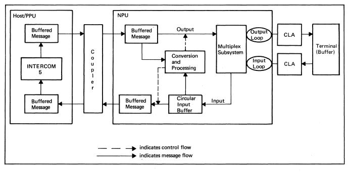
Figure 2-1. Simplified NPU Buffered Transfers
