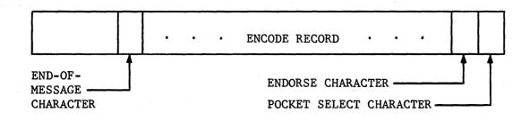
Figure 4-10. Encoder Controller Buffer
