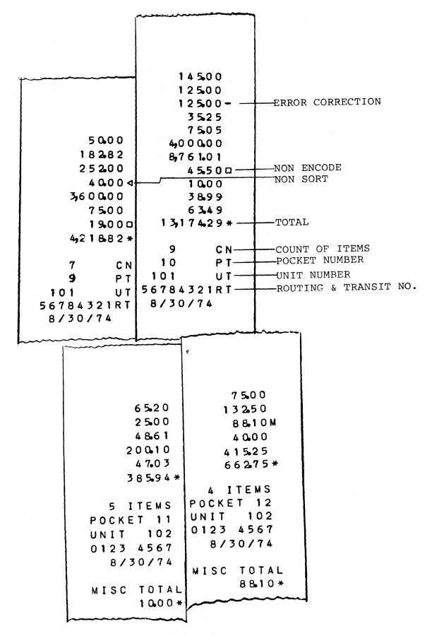
Figure 4-13. Example Prints of the Two-Tape Detail Lister COLUMN
