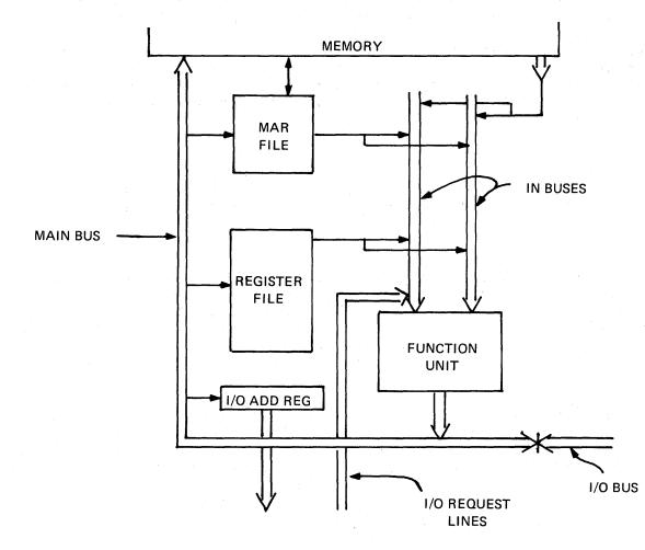
Figure 2-3. General Processor Architecture
