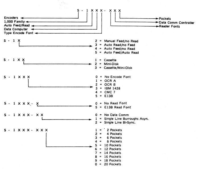
The additional specifications required for the S 1000 system are as follows:
