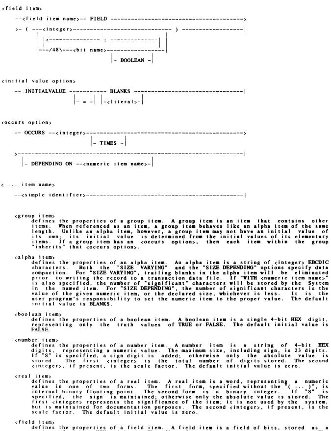
defines the properties of a field item. A field item is a field of bits, stored as a string of 4-bit HEX digits. The first form will accommodate <integer> bits. The <integer> cannot exceed 48. The second form will contain up to 48 bits, each individually accessible as a boolean value by using the appropriate <br/>bit name>. The
