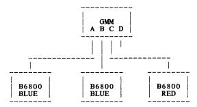
Ports A and B are tightly-coupled as the two-processor BLUE group. Port C is the one-processor RED group. No matter what happens to one of the two groups, the other should not be affected. The RED group need not even run on the same MCP as the BLUE group. RED and BLUE are autonomous.
