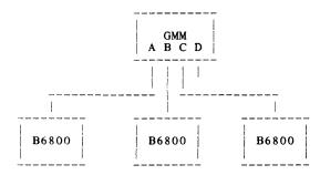
This installation has been running in the default mode (i.e it has been running as a 3-processor tightly-coupled installation) because no groups have ever been specified. Now, the installation manager wishes to assume the configuration of example 3:
