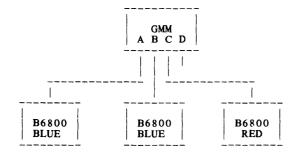
Each B6800 has local memory (see D-note D2861). In this example, assume that each local memory has  $32\ 16K$  memory modules. Therefore, mods 0-31 are local to each processor. Also assume that there are  $32\ 16K$  modules of global memory. An attempt by any processor to reference mods 32-63 will be a global memory request.
