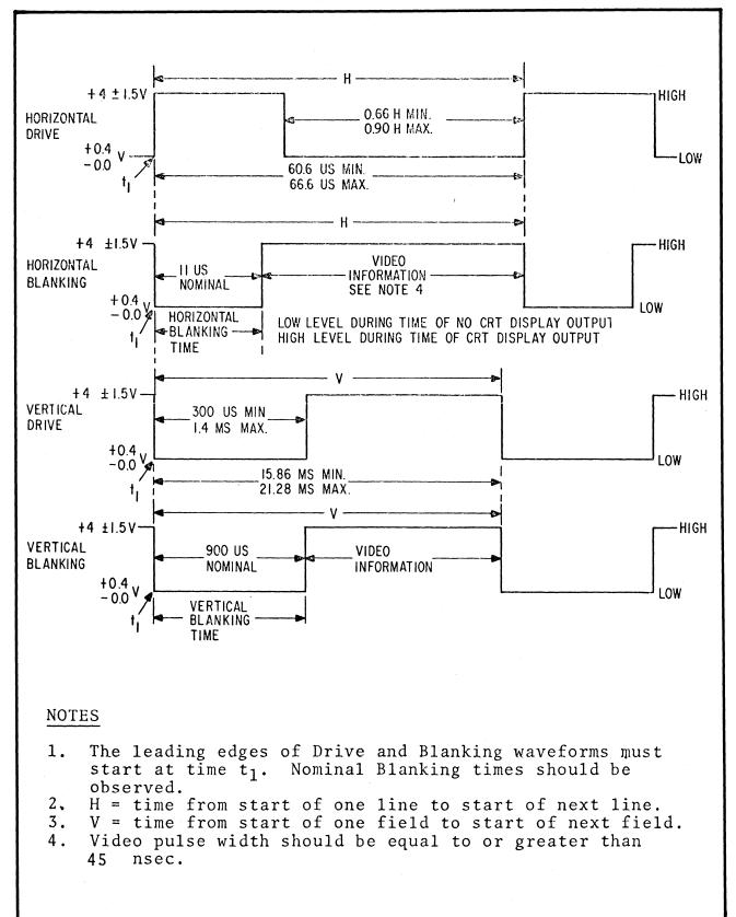
Fig. 1 Synchronization and Blanking Generator Waveforms for the TTL Series Data Display Series.
