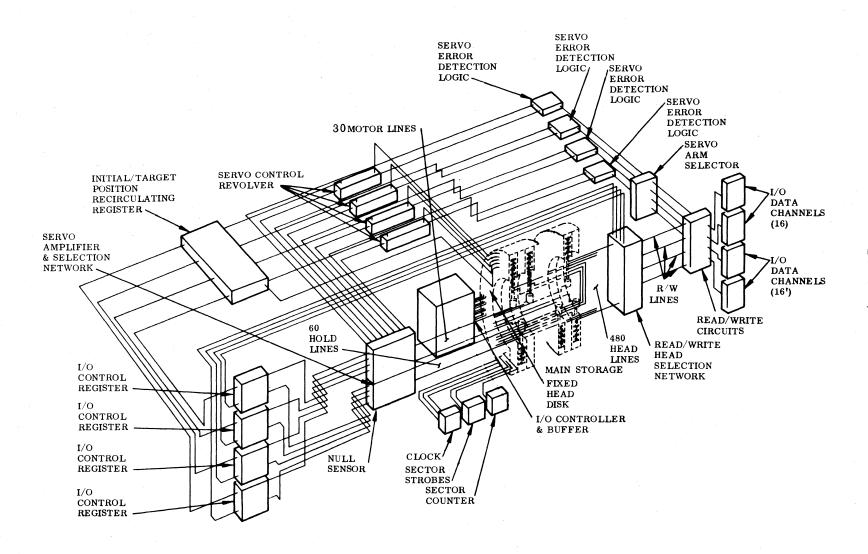
Figure 2. Functional Schematic of 30-Arm Digital Disk File
