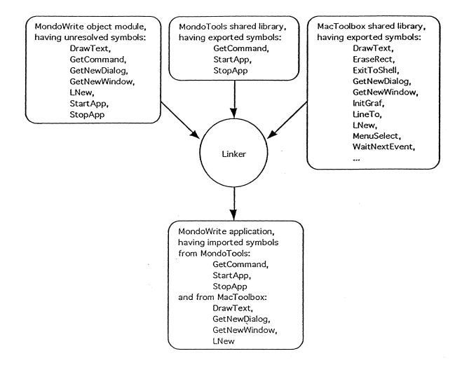
Figure 2. An illustration of export and import handling by the linker.
