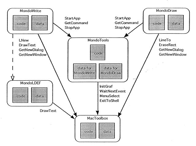
Figure 3. An illustration of application, shared library, and extension fragments in operation.
