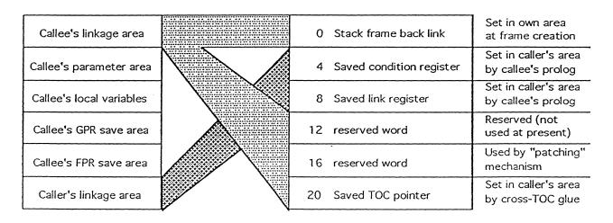
Figure 5. Details of stack frame linkage area
