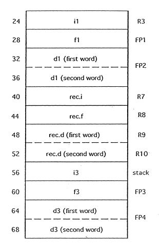
Figure 8. Register mapping example
