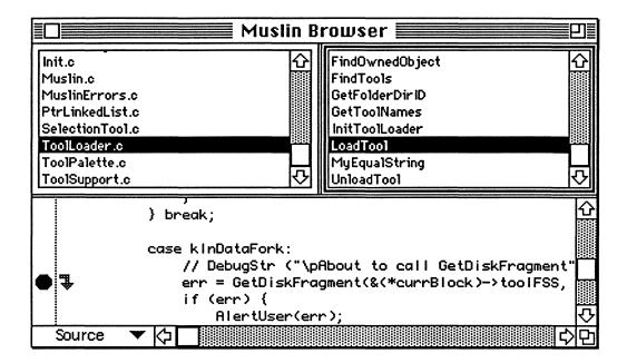
The "crooked arrow" indicates that the next "step" command will step into the specified call. (GetDiskFragment.) Since stepping into this routine would involve looking through assembly code, select the "step over" command at the right end of the palette, or set a breakpoint on the next executable line and run. (You may need to click "step over" several times to get out of the breakpoint.)
