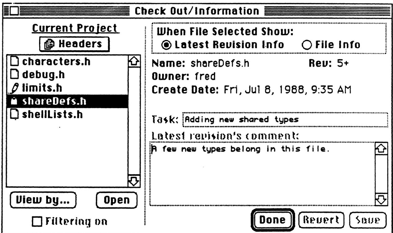
Figure 8 - Project information in the "CheckOut" window.
