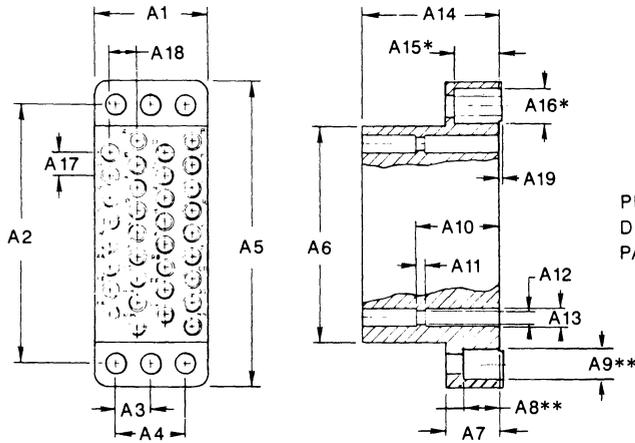
PIN BLOCK AND SOCKET BLOCK ARE DIMENSIONALLY THE SAME, SEE NEXT PAGE FOR CAVITY IDENTIFICATION.
