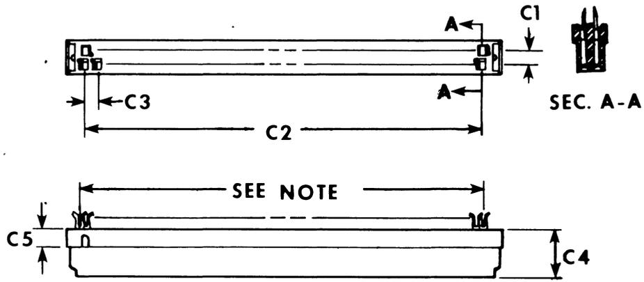
NOTE: 60 contacts on 0.050 inch (1.27 mm) staggered spacing = 2.950 inches (74.93 mm)
