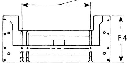
NOTE: 26 contacts on 0.100 inch (2.54 mm) spacing = 1.200 inches (30.48 mm)
