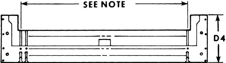
NOTE: 60 contacts on 0.100 inch (2.54 mm) spacing = 2.90 inches (73.66 mm)
