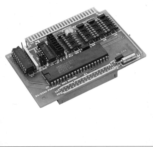
The Am94/0350 Parallel I/O (PIO) Module is an 8-bit singlewidth SBX module which provides the designer a low-cost, high-performance method for adding incremental I/O capability. The module consists of an 8255A-5 Programmable Peripheral Interface (PPI) and sockets for line drivers and terminators which provide for 24 lines of configurable parallel I/O.
