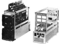
supply. It furnishes  $\pm 5$  and  $\pm 12VDC$  (regulated) MULTIBUS voltage requirements. The power supply module, MULTIBUS backplane, input panel, cooling fans, and metal frame are integrated into a compact trim design for use in industrial chassis and for benchtop use (see Figure 2).
