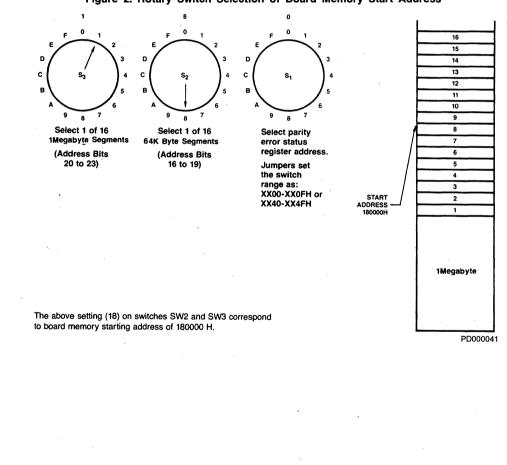
Figure 2. Rotary Switch Selection of Board Memory Start Address
