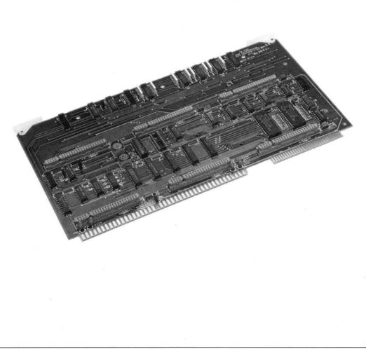
The Am94/2000 SBX Motherboard is a MULTIBUS-compatible board which can add SBX capability to any MULTIBUS system. Six SBX connectors are provided to support singlewidth and double-width modules not requiring DMA. Am94/ 2000 features include MULTIBUS address decoding and data buffering, MULTIBUS-SBX timing reconciliation, and two interrupt controllers.
