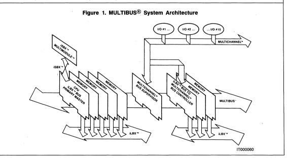
defined by the iLBX Bus Specification consist of 16 data lines and 24 address lines.
