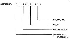
$\text{CS}_0/\text{CS}_1,\,\text{MA}_0,\,\text{MA}_1,\,\text{MA}_2$  are sent to the SBX module and used as needed.
