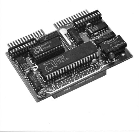
The Am94/1530 is a programmable, dual channel serial communications module for the SBX bus. The module adds two RS-232C serial channels to any host board which includes an SBX bus compatible connector. This enables the designer to add incremental I/O capability at lower cost and higher performance than alternative methods.
