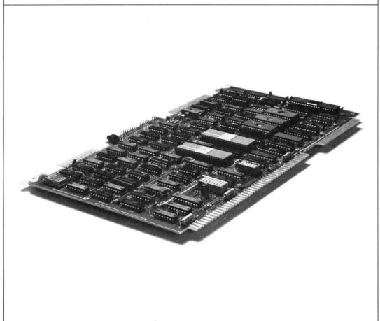
The Am95/6120 Intelligent Floppy Disk Controller (IFDC) includes an 8085A Microprocessor, an FD1793 Floppy Disk Controller, 1K bytes of high-speed static RAM, a 9517A DMA Controller, 3K bytes of EPROM firmware and five interfacing mailbox registers. The functional diagram in Figure 1 shows the architecture of the board.
