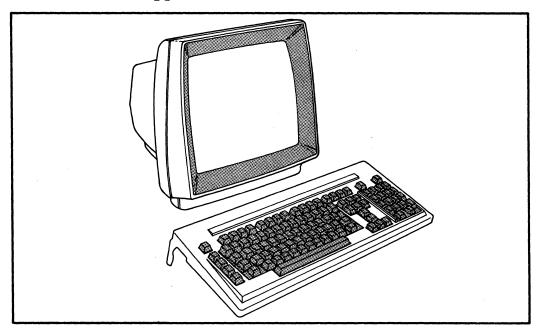
If you do not need "hard copy," which means a printout on paper, you can display the results of your computer session on the terminal. For example, you enter text from the keyboard which displays on the screen. You have a program that formats the text, but before you have the text printed on paper, you display the rearranged text on the screen exactly as it will appear on paper. Suppose you find an error. You can correct it via the terminal and prevent having to throw away the first printout.
