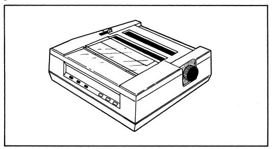
Print quality may or may not be important. If you are producing text that is to be "camera ready" for printing, you need a letter-quality printer. (Characters are produced by one stroke of a letter template against the ribbon as on a typewriter.) If you simply need readable copy, which can also be high quality, a dot-matrix printer is a less expensive option. (Characters are produced by a series of points that press against that ribbon to make up the letter.)
