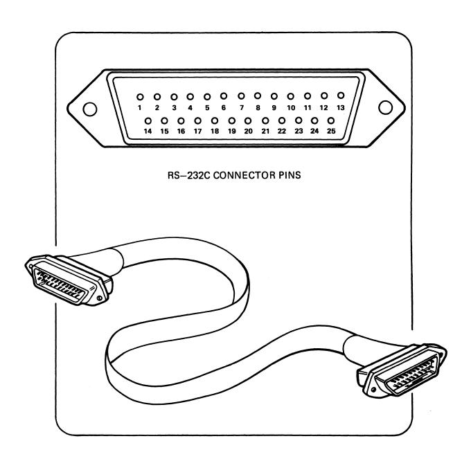
Figure C-1: Male Connector, RS-232C Cable
