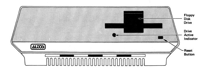
Figure 6-1: Altos 58# Front and Rear Panels
