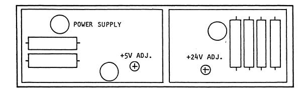
Figure 4-2. Adjustment Potentiometers
