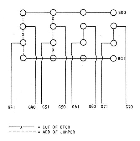
Figure 2-5. PDP-11 Interrupt Priority Level Jumpers
