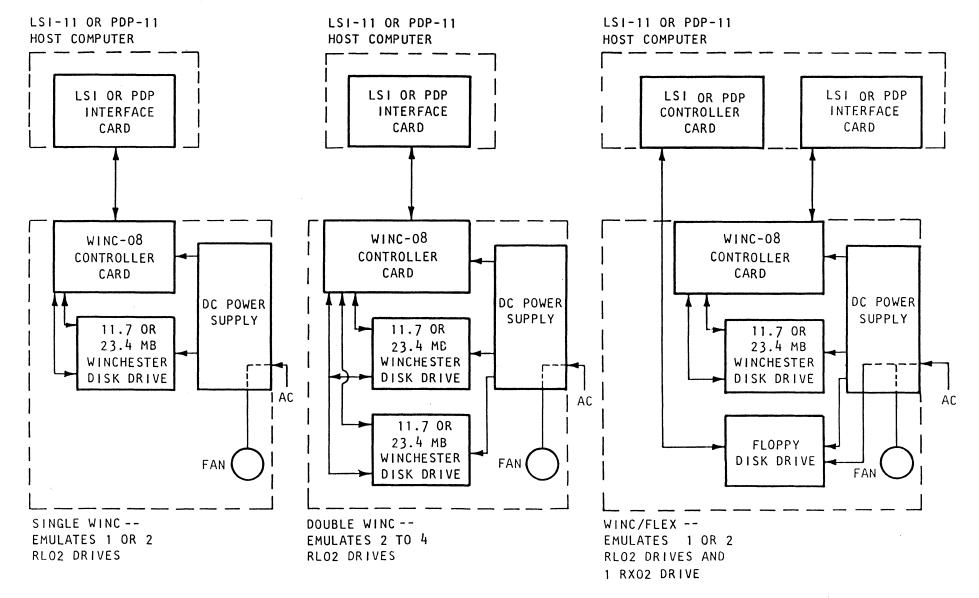
Figure 1-2. WINC-08 Standard Configurations
