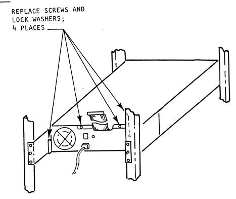
Figure 2-1e. Top/Sides Installation
