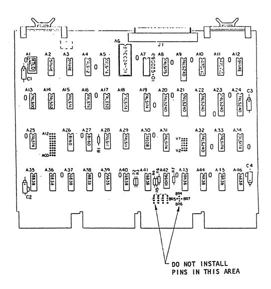
Figure 5-7. PDPII Interface Assembly
