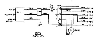
Figure 5-5. Rear Panel Assembly (Sheet 3 of 4)
