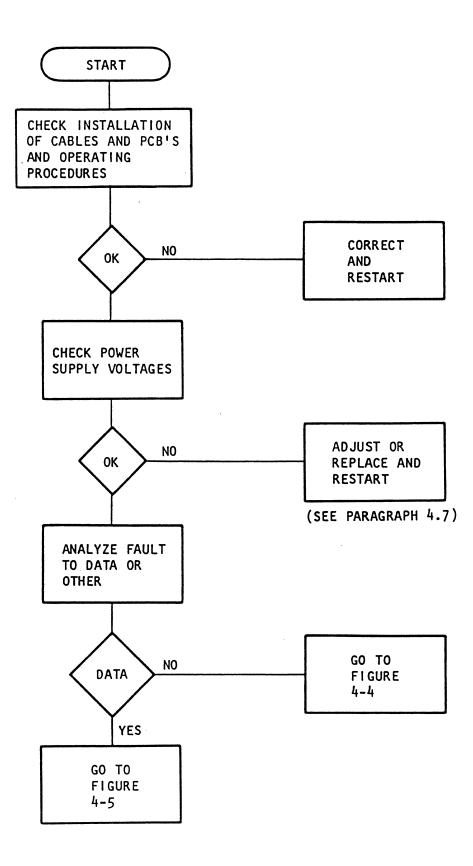
Figure 4-3. Basic Checks
