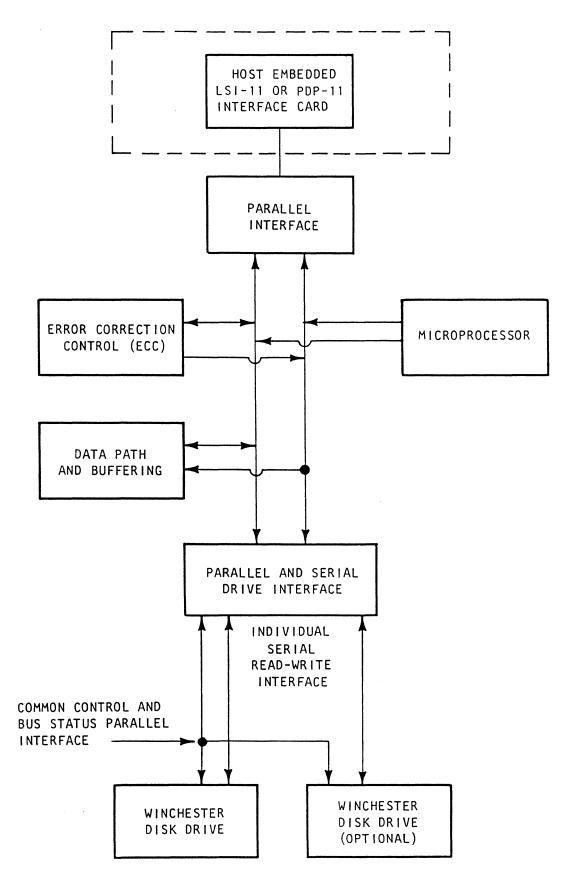
Figure 1-1. Typical WINC-08 Functional Block Diagram
