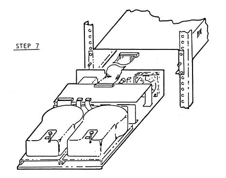
Figure 2-1d. Assembly into Top/Sides
