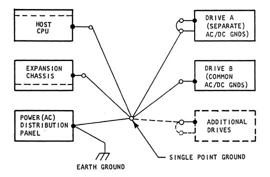
Figure 2-2. System Grounding Diagram
