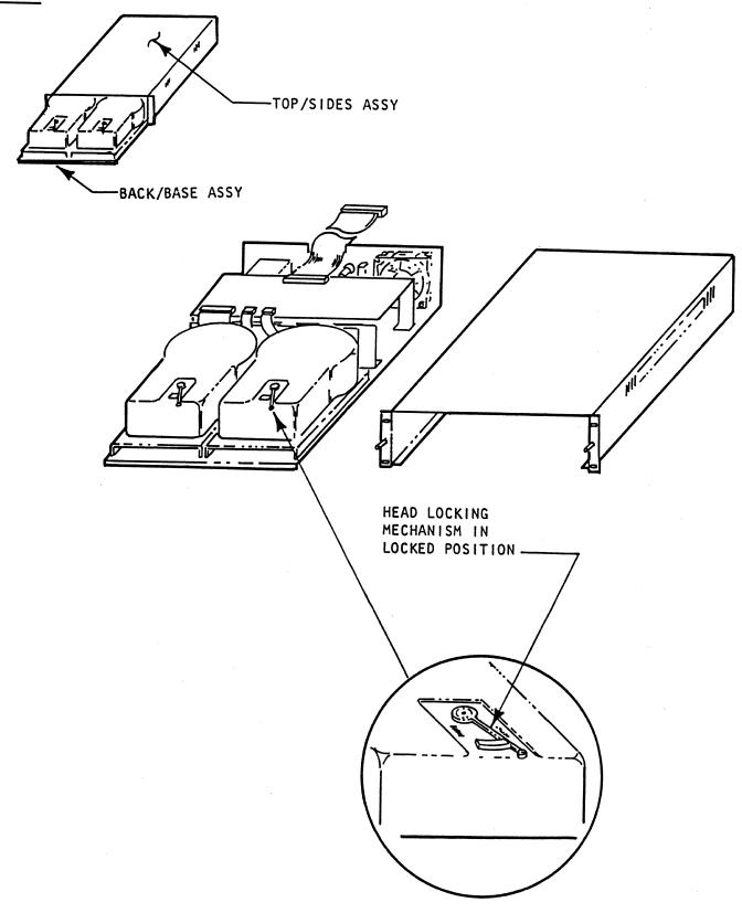
Figure 2-1b. Winchester Drive Head Lock Mechanism
