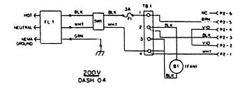
Figure 5-5. Rear Panel Assembly (Sheet 4 of 4)
