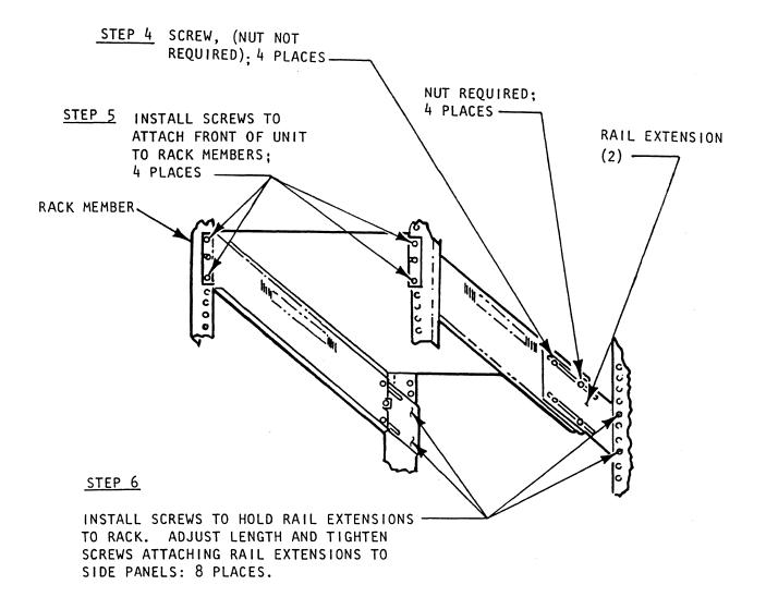
Figure 2-1c. Rack Installation
