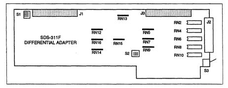
Figure 1-1. SDS-311F Differential Adapter PCB
