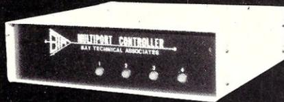
**BTA's MODEL 524 MULTI-PORT CONTROLLER** is a code activated one to four serial port expander — but that's not all since it has separate and independent UARTS, buffers and handshaking each port can operate with a different configuration, i.e. different baud rates, stop bits, etc. These features also permit two or more devices to communicate with the 524 simultaneously.
