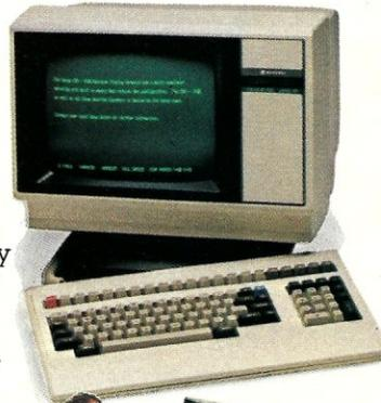
Parallel and RS-232C interface. Partial scroll and block mode. 8 user programmable keys.
