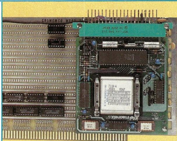
*Bubble Memory S-100 board showing Intel subsystem.*
