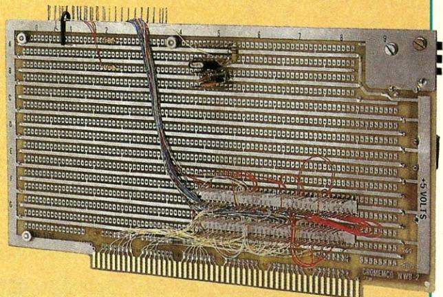
Bubble Memory S-100 board, wiring side, showing clock crystal (top center).
