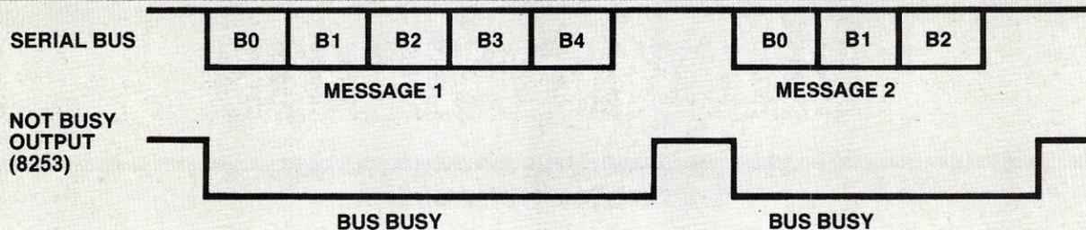
Figure 6. Serial bus timing.
