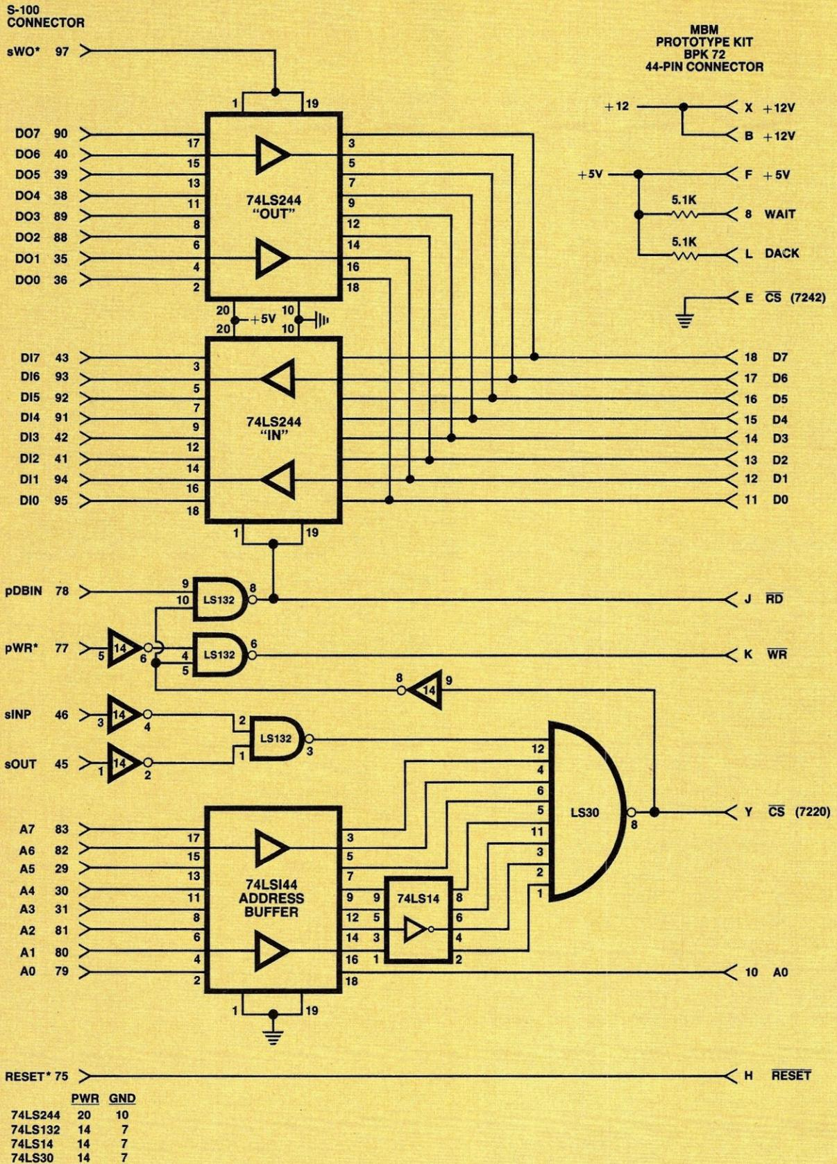
Figure 2. Bubble memory system interface.
