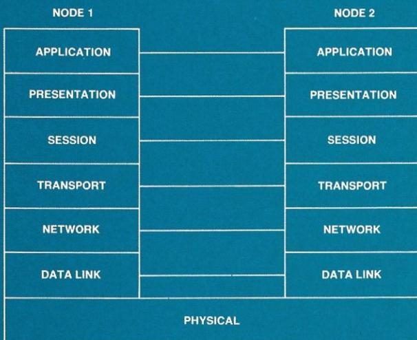
Figure 1. Logical Connection between layers.
