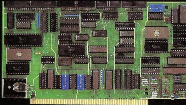
A hard disk and cartridge tape controller together on one board? Magic? Not really. It's Teletek's HD/CTC. The hard disk and cartridge tape drive controller provide the support necessary to interface both rigid-disk drives and a cartridge tape deck to the S-100 bus.
