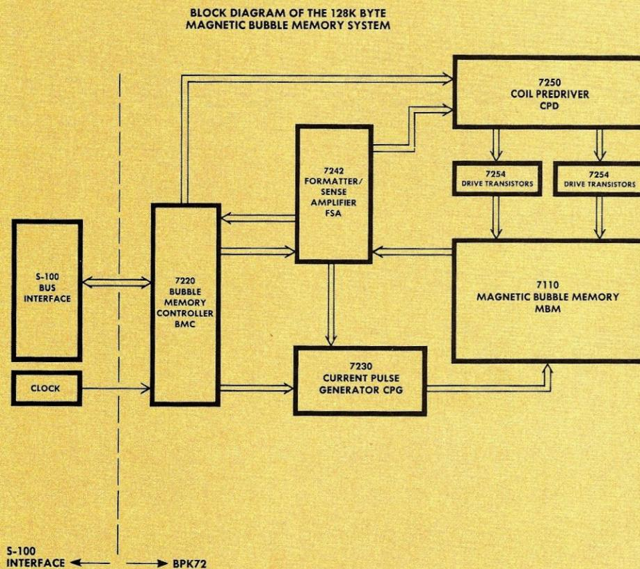
Figure 1. Bubble memory system, block diagram.
