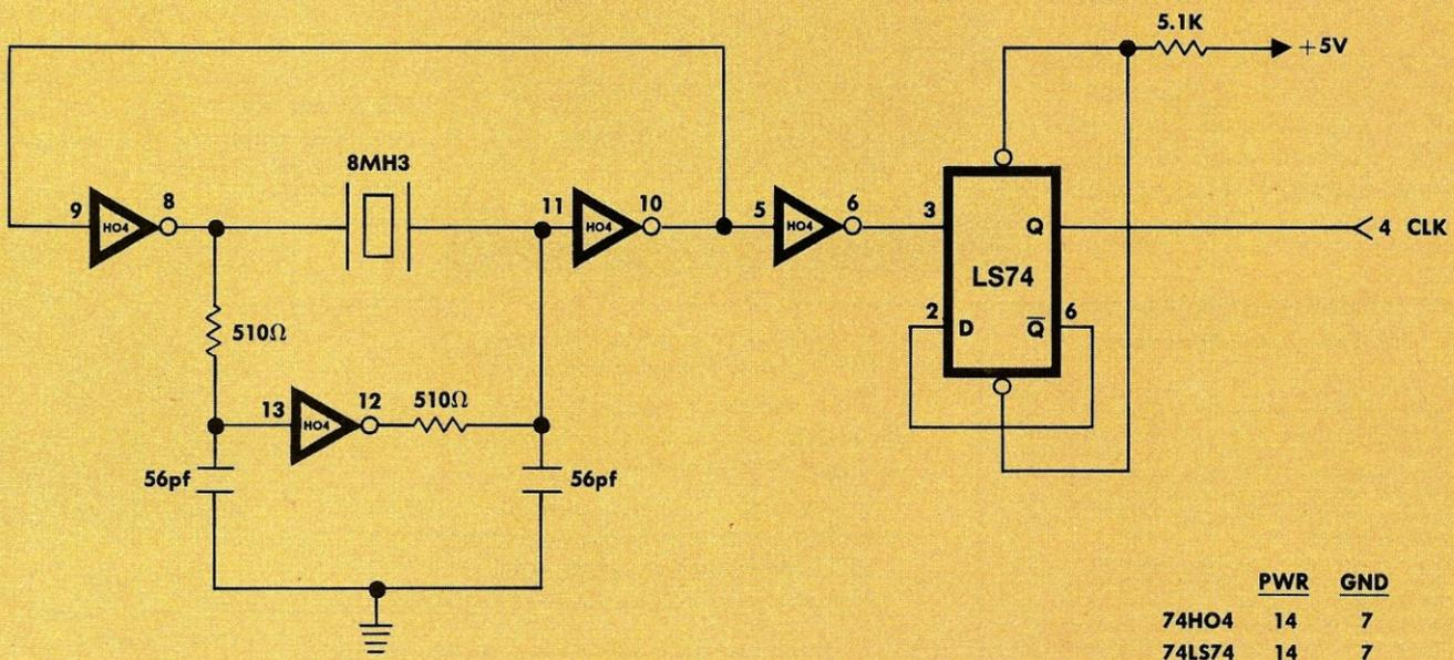
Figure 3. Clock circuit, copied from INTEL application NOTO (AP119) microprocess interface for the BPK72, June, 1981.
