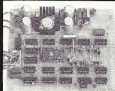
**- INTERFACES THROUGH ONE 8 BIT INPUT PORT AND ONE 8 BIT OUTPUT PORT. 16 WIRES - NO SPECIAL HANDSHAKE LINES.**
