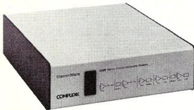
StationMate provides three data ports with standard RS-232C connectors. The model gives a fourth (remote) user access to the system. This means that the user can establish a remote workstation at home or at any other location and have full access to the network.
