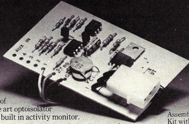
Our DCU is the original Drive Control Unit that turns floppy drives off during periods of inactivity by using a state of the art optoisolator with zero crossover control and built in activity monitor.
