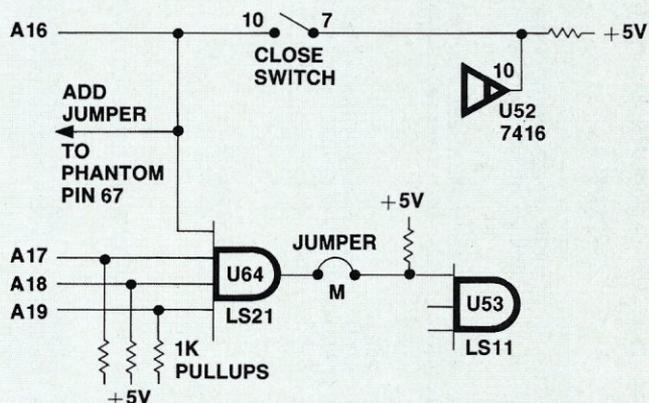
Figure 2. VIO modifications for operation with CCS 2422: jumper M, close switch 7, add pullups to A17 through A19.
