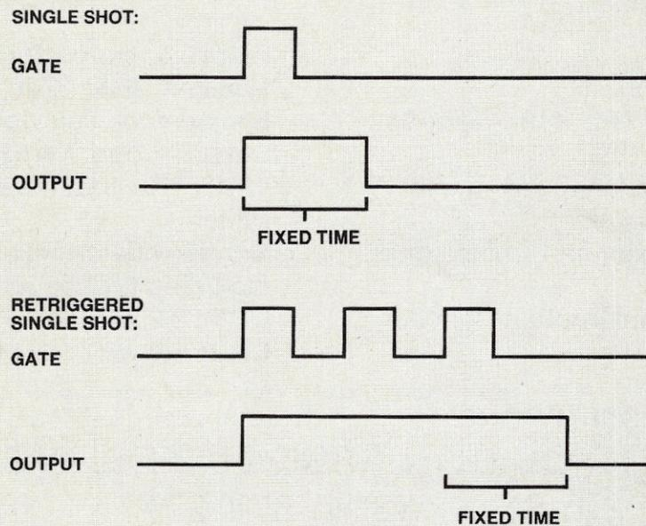
Figure 5. Single shot timing diagram.
