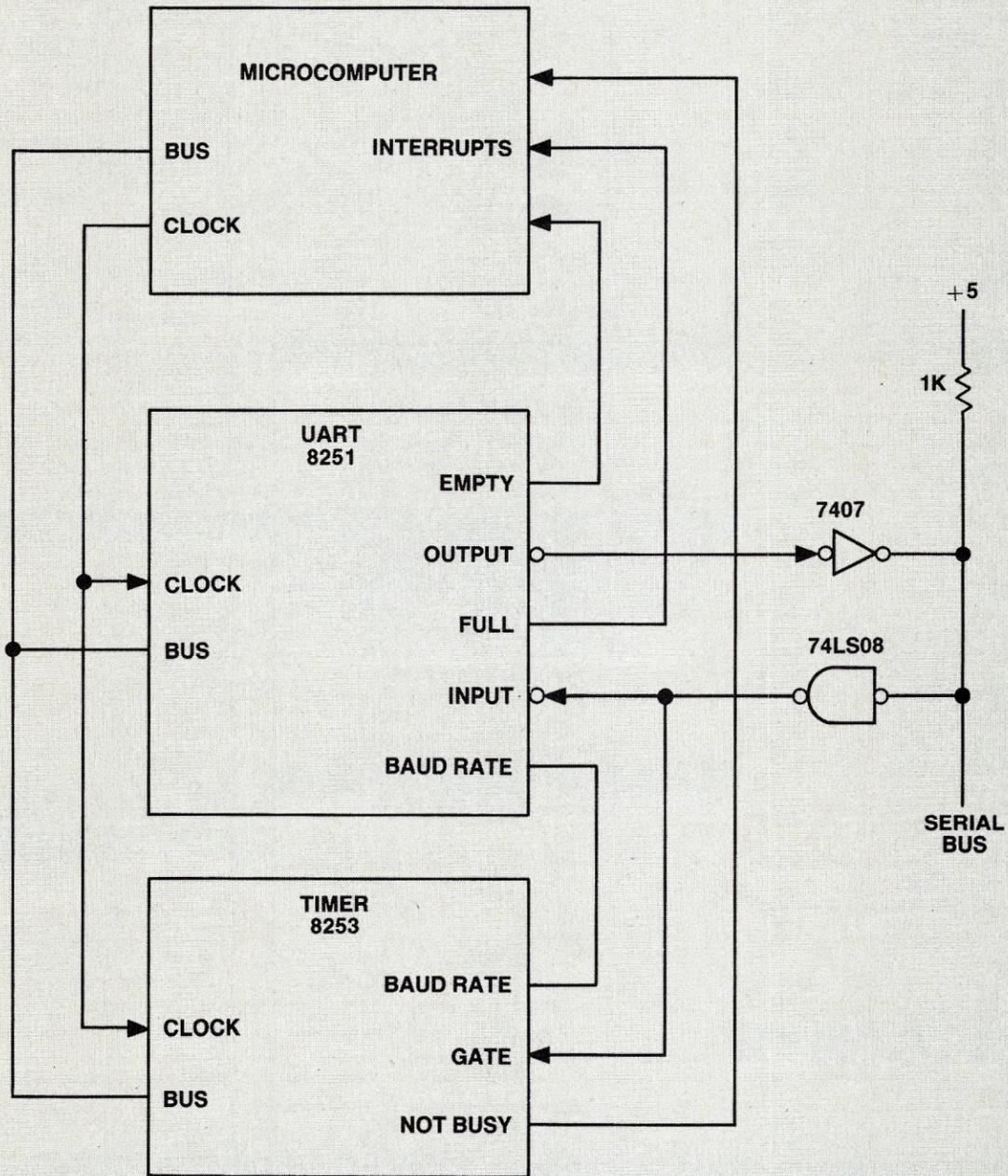
Figure 3. Serial bus interface.
