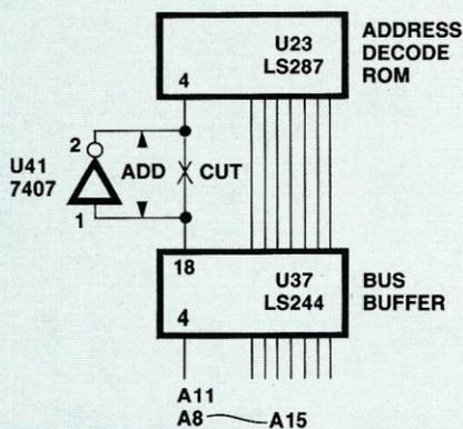
Figure 1. F800 modification to CCS 2422 uses spare inverter of U41.
