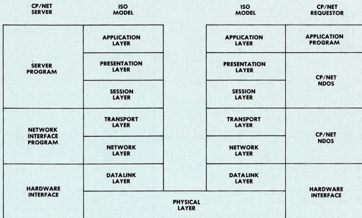
Figure 2. CP/NET and the ISO network model.
