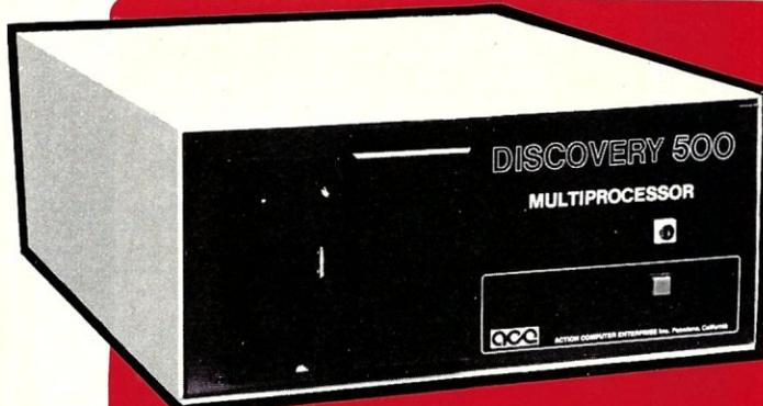
The DISCOVERY 500, a fully integrated desktop computer with 5 1/4" hard and floppy disks, supports up to 7 users. It is the ideal, low cost turnkey business system. The full size DISCOVERY supports up to 16 users with a wide variety of disk and tape subsystems. And remember, all DISCOVERY users have their own dedicated memory and 8-bit or 16-bit CPU, running CP/M-80\* or CP/M-86\*. Action's own multiuser multiprocessor operating system, the **dpc/os**† makes it easy.
