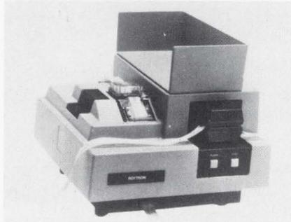
6, 7 or 8-level paper tape in 1", 7/8" or 11/16" widths. \$2000 with integral power supply. *Litton Automated Business Systems, Pine Brook, NJ.*
