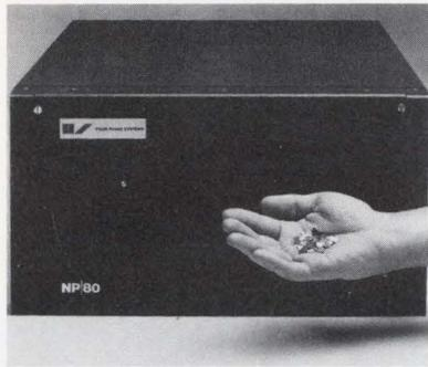
*Four-Phase Systems' new NP/80 Network Processor. The heart of the NP/80 is a powerful 16-bit computer with 500 nanosecond cycle time and up to 256K bytes of MOS/LSI memory. The hand in the foreground contains all the 16K-bit RAM chips needed for a 256K byte memory including error correction. These devices, designed and manufactured by Four-Phase, will occupy a single printed circuit board when assembled.*
