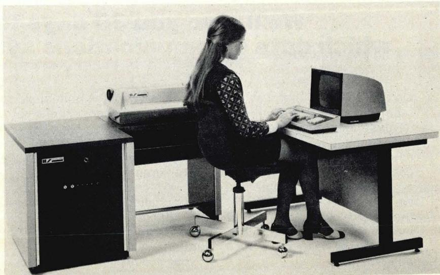
An excellent example of the new, multi-mode terminal systems for decentralized operations is Four-Phase Systems' Model IV/40 Remote Intelligent Terminal System. The IV/40 features a 72 Kbyte LSI processor with integrated cartridge disc drive; supports up to 16 CRTs and 16 printers for source data entry, remote batch processing, IBM 3270/2260 emulation, and custom network applications. Four-Phase was one of the first companies to appreciate the potential of intelligent terminals.
