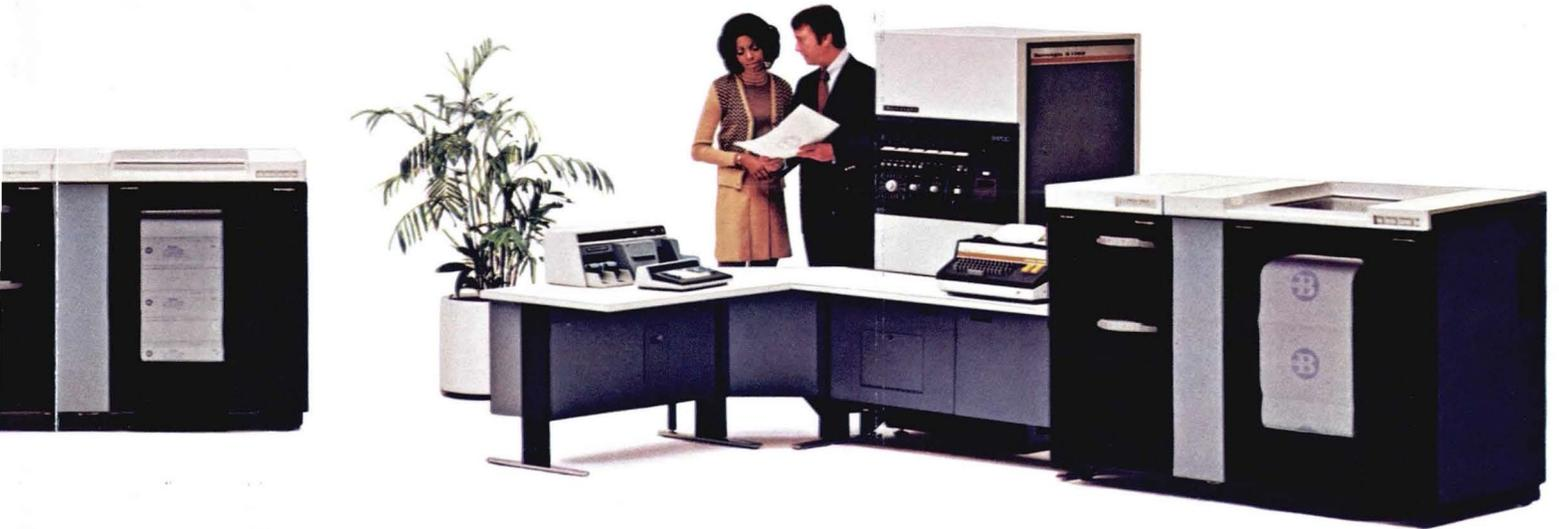
**B 1700 SYSTEMS** satisfy business management requirements and can serve engineering and production, as well. Like Burroughs larger scale computers, the B 1700 Systems operate on multiple data processing jobs at the same time. Their advanced features include "virtual memory" operation for high system efficiency, and a Master Control Program for system self-management.
