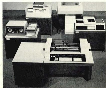
Accounting Computer/Small Business Computer. The NCR 399 straddles the dividing line separating an accounting computer from a disc-based small business computer. The unit record oriented 399 offers a complete range of magnetic ledger card, line printer, tape and card options, and can come with auxiliary disc “platter” storage.
