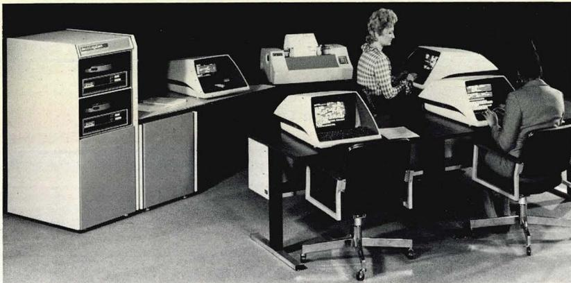
OEM-Type Small Business Computer. The DEC Datasystem series of small business computers provide full hardware and operating system (OS) capabilities, leaving the turnkey systems house or user the task of developing business applications packages. These OEM-type small systems are offered by most of the major minicomputer mainframe manufacturers.
