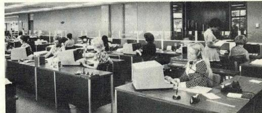
In typical business situation Hewlett-Packard Terminal Control System software gives many terminals simultaneous, interactive exchange with a central disc-resident data base as large as 47 million bytes.
