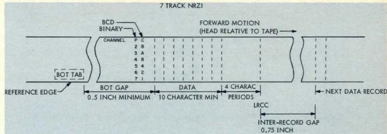
Figure 1 • 7-Track NRZI Format (courtesy of Peripheral Equipment)
