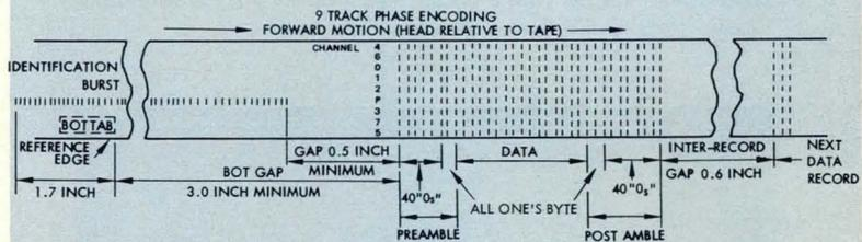
Figure 3 • 9-Track Phase Encoded Format (courtesy of Peripheral Equipment)
