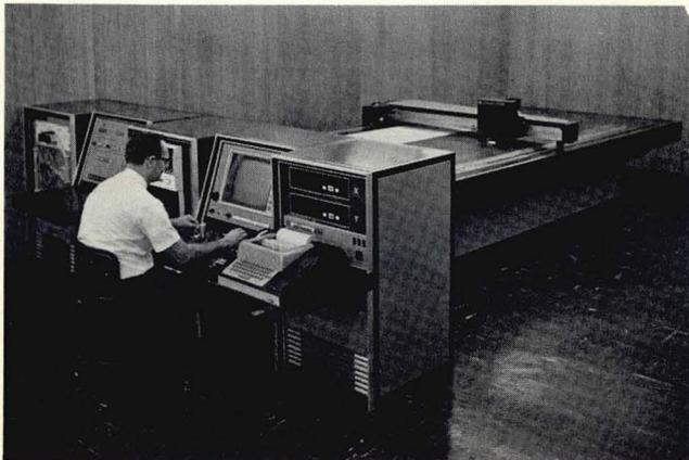
Figure 2 • Actron Industries/Tridea Products Division's ALTAPE/ALDRAFT Systems, an automatic line-following graphic digitizer/plotter system.
