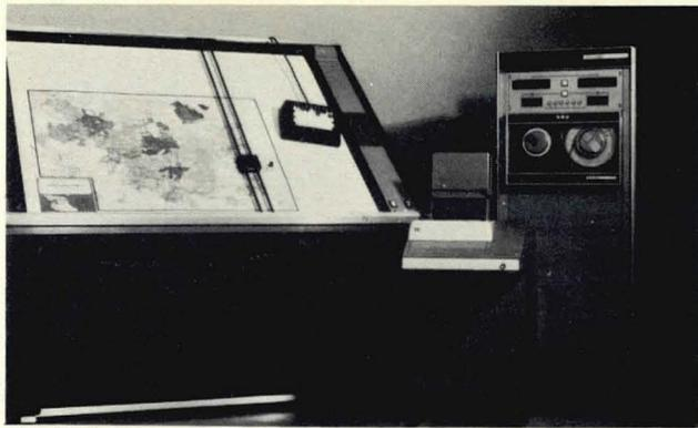
Figure 5 • The Model 785 Graphic Data Digitizer, Calma's large bed system which outputs onto seven- or nine-track magnetic tape.
