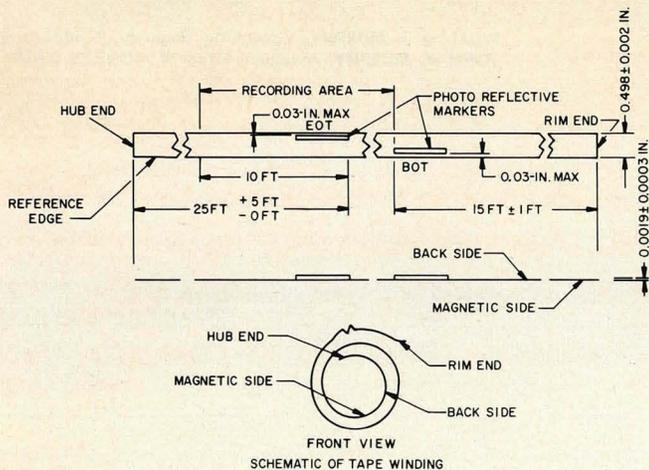
Figure 4 • Tape Markers, Recording Area, and Tape Wind (courtesy of USAI)
