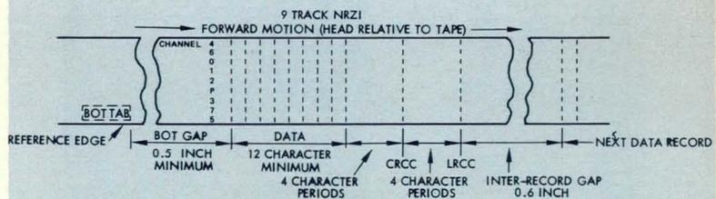
Figure 2 • 9-Track NRZI Format (courtesy of Peripheral Equipment)
