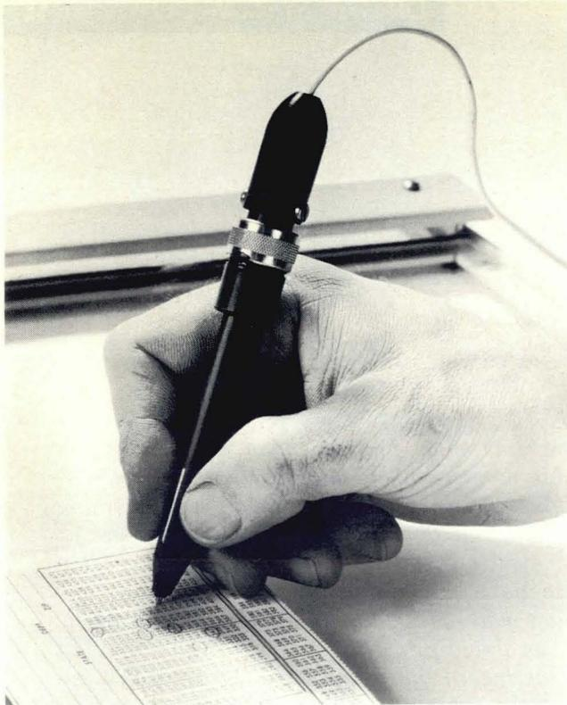
Fig. 1—A Graf/Pen being used to mark, and enter data simultaneously from, a MODERN DATA Reader Service Card. The metal strip built into the side of the tablet at the right of the card (top on photo) senses sound waves generated by a spark produced at the pen's tip. Another strip, not shown in this close-up photo, is built into the tablet above the card.
