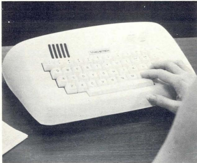
A Wavetek audio-response terminal being used as a desk-top source data entry station.
