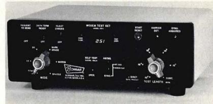
The modem output is received by the test set and a self-synchronizing circuit compares the pattern received to that which should be received. If a difference is detected, a numerical counter is incremented. *Bowmar/ALI, Acton, Mass.*
