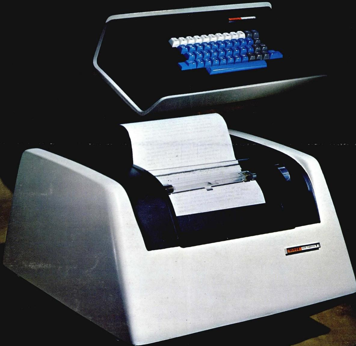
The REPCO 120 is a low-cost, solid state impactless printer designed to interface with all CRT terminals, minicomputers or other remote data terminals. It operates asynchronously at speeds to 120 characters per second, 80 characters per line, 5 lines per inch vertically. It will handle serial or parallel data of 64 character standard ASC II code. When interfaced with a modem or acoustic coupler, it can be used
