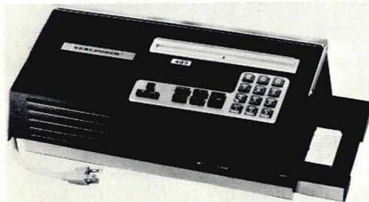
tion, etc., and from its integral keyboard. It can also control other devices, such as adding machines, through self-generated output signals. All control functions including tab (skip), space, hold, and return may be actuated from remote signals. Alpha and numeric data in up to four hole combinations are punched at twelve characters per second. *Varifab, Inc., Old Greenwich, Conn.*
