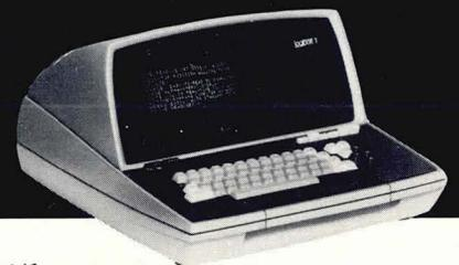
It's the Logiport/1, the first truly portable, remote-access CRT terminal with integral acoustic coupler. Available immediately, it's incredibly priced at under \$3,000. Compact design fits easily on desk top. Easy-to-read, 32-character-line, alphanumeric display. Interactive Terminals Corporation, 197 Albany St., Cambridge, Massachusetts 02139. A subsidiary of The Bendix Corporation.
