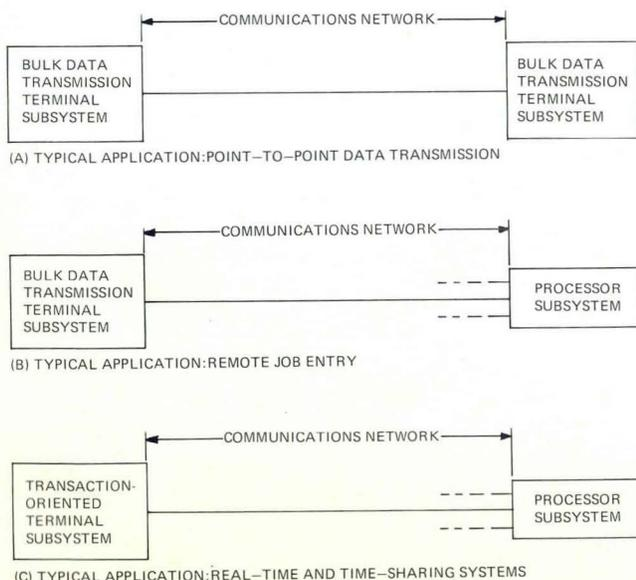
Fig. 8 — Classification of data communications systems for performance estimation purposes.
