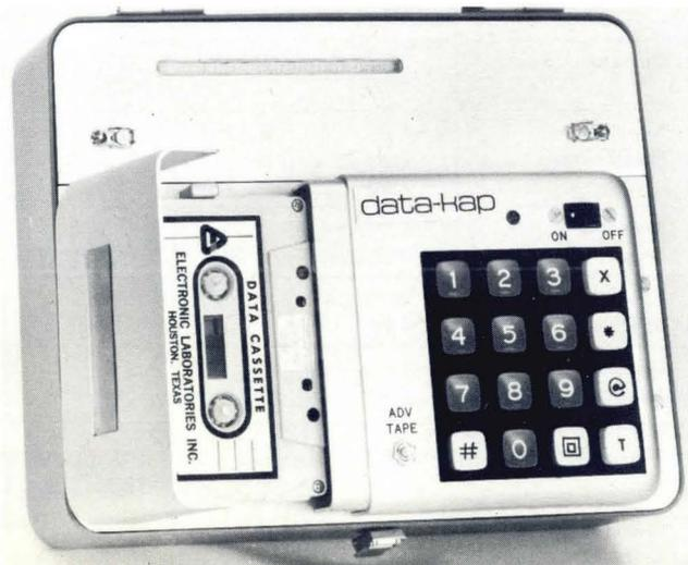
Fig. 4 — The "data-kap" Model 806 from Electronic Laboratories, Inc. is completely portable (battery-powered) and records numerics on magnetic tape cassettes. An optional, built-in strip printer provides immediate data verification as well as a hard copy record.
