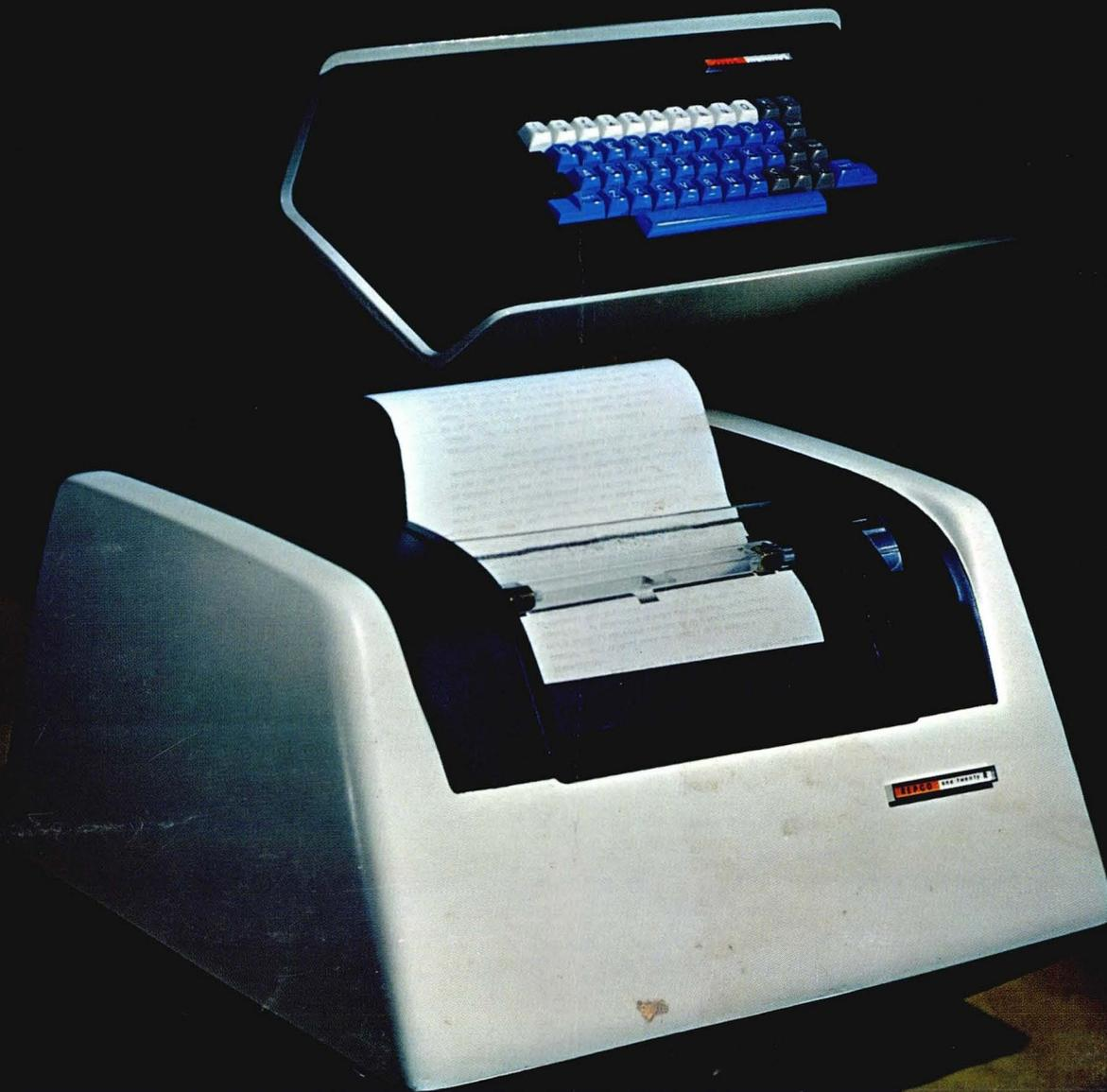
The REPCO 120 is a low-cost, solid state impactless printer designed to interface with all CRT terminals, minicomputers or other remote data terminals. It operates asynchronously at speeds to 120 characters per second, 80 characters per line, 5 lines per inch vertically. It will handle serial or parallel data of 64 character standard ASC II code. When interfaced with a modem or acoustic coupler, it can be used
