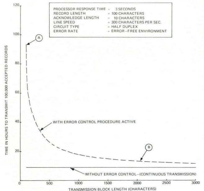
Fig. 3 — Effects of error control procedure.
