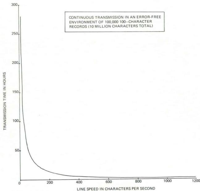
Fig. 2 — Minimum transmission time versus line speed.
