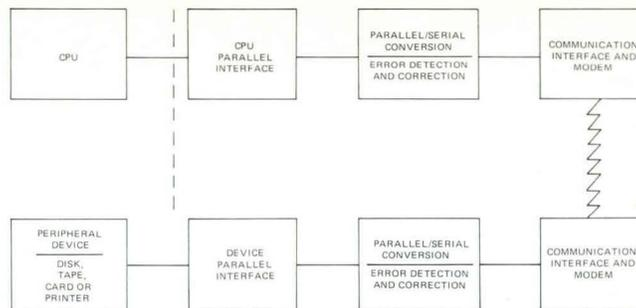
Fig. 1—Block Diagram of Paradyne's PIX-600 Parallel Interface Extender.
