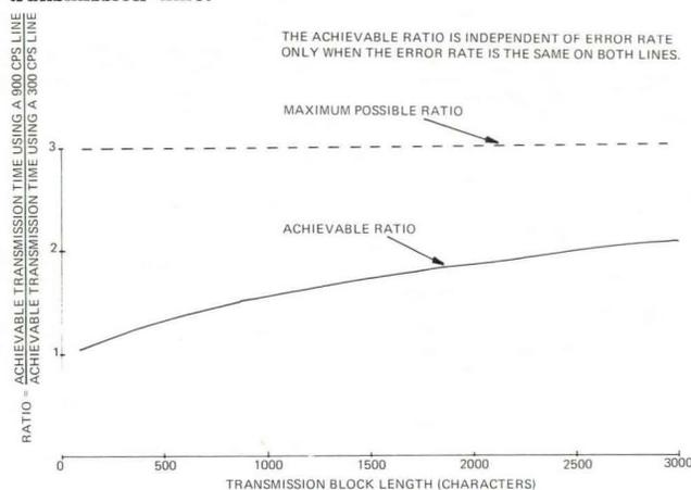
Fig. 7 — Effect of line speed on achievable transmission time.
