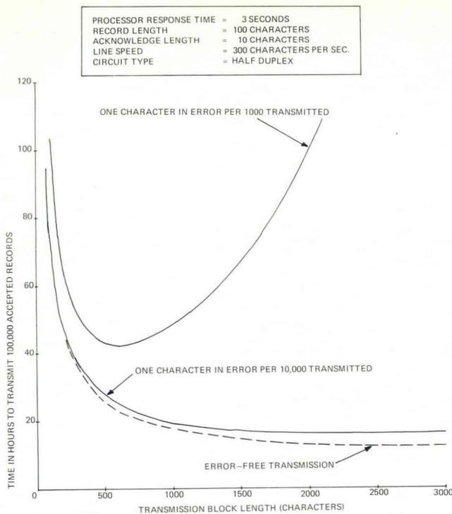
Fig. 6 — Effect of transmission block length on achievable transmission time.
