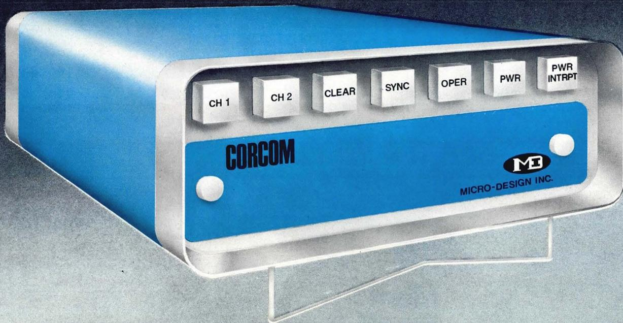
... An advanced system of digital error detection and correction... specifically designed to protect your data communications channels from costly gremlins and garbling.
