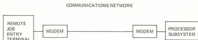
Fig. 1 — Major components of a remote job entry system.
