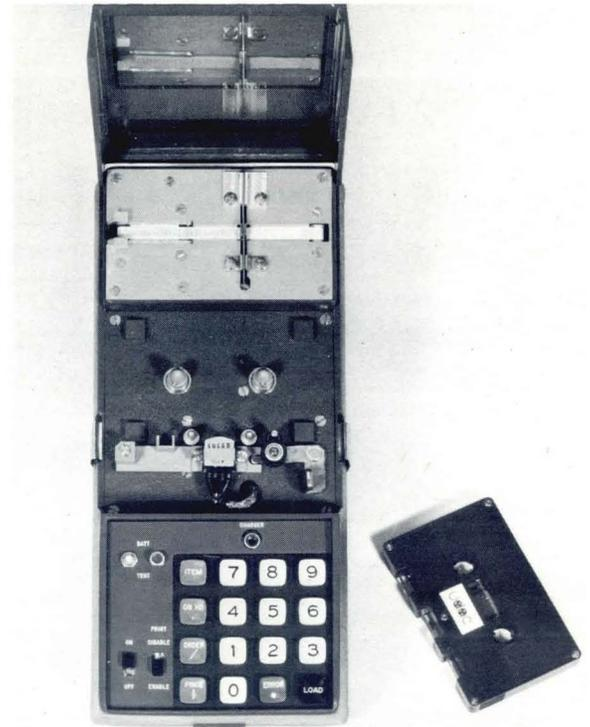
Fig. 5 — The UDAC Model 5021 from Universal Data Acquisition Co. is a battery-powered alphanumeric device which records on magnetic cassettes and an integral strip printer. Used in conjunction with a UDAC transmitter, receiver/converter, and modem, it constitutes a complete data acquisition system.
