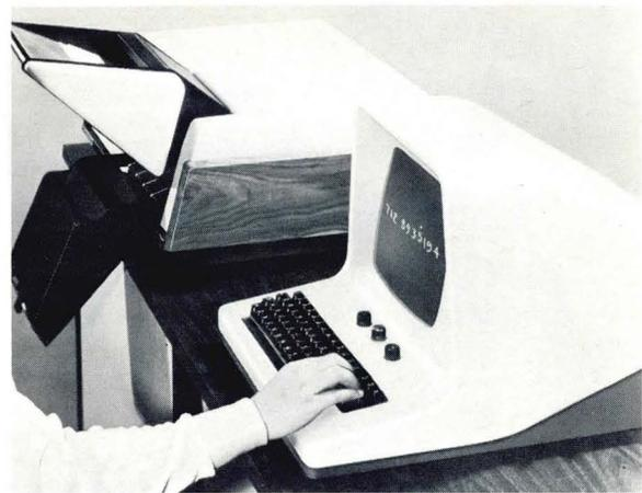
Fig. 1 Cognitronics' System 70 Optical Character Reader
