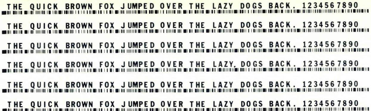
Fig. 2 Sample of coded font scanned by Datatype Corp.'s Dataflow Optical Reading System
