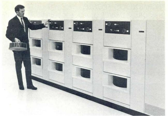
The IBM 3330 disk-pack storage system, available in 2-, 4-, 6-, or 8-drive configurations with capacities of from 1600 to 6400 megabits, and a transfer rate of 6.45 megabits/second.
